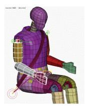
Figure 3.2: Positioning the dummy using ANSA 12.01
