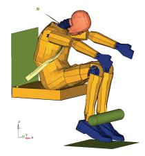
Figure 3.1: HyGee 25g Forward Impact Pulse
