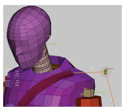
Figure 1.1 – Attachment of the restraint system to the B-Pillar
