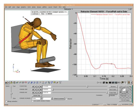
Figure 5.0: Post-Processing with HyperView v7.0
