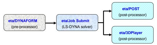
Figure 1: Components of eta/DYNAFORM solution package.
