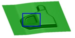
Figure 5.58 Cam formed feature
