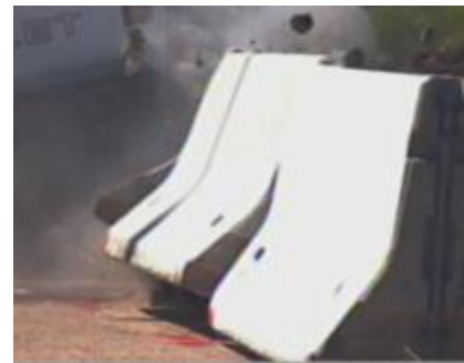
(b) Lifting of barriers observed in modified simulation and test
