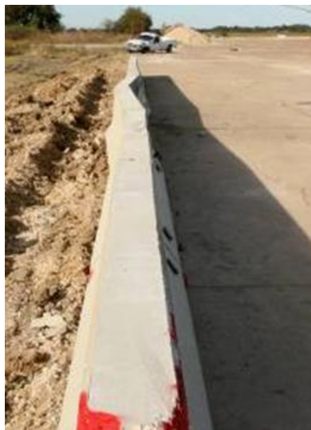
Figure 7 Pinned-down F-shaped temporary barrier after testing.
