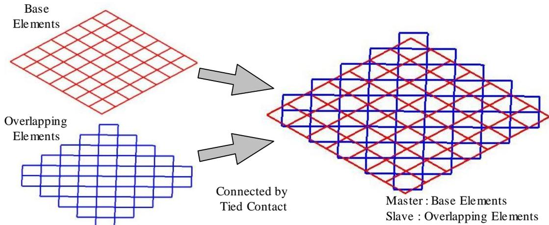
Figure 3. Tied overlapping shell technique.
