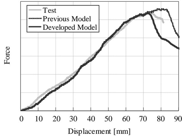
Figure 10. Comparison of force versus displacement during roof strength test between test and numerical simulation.
