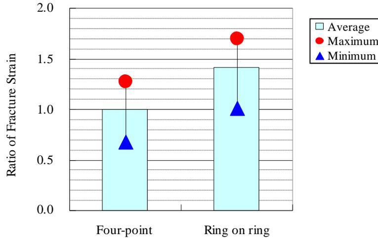
Figure 7. Comparison of fracture strain between edge and in-surface.
