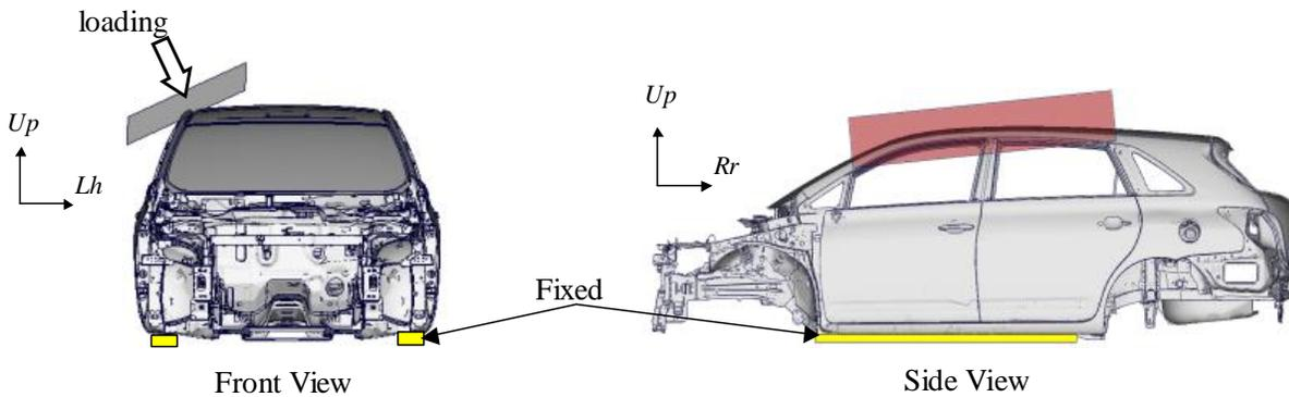
Figure 8. Roof strength model boundary condition.
