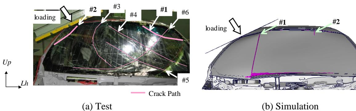
Figure 1. Comparison of glass crack propagation paths after roof strength test between test and numerical simulation.
