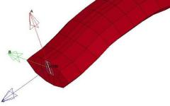
Fig. 3 FE model of an individual yarn. Stiffness matrix of the material is a symmetric one.
