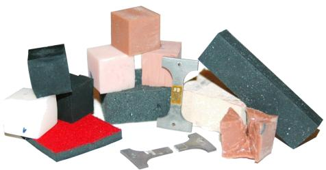
Figure 3: Material specimens of the WorldSID 50%.
