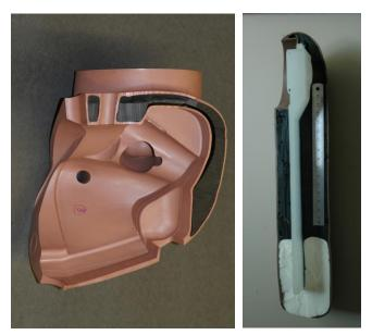
Figure 2: Cut through a new arm and pelvis flesh of the WorldSID 50%.
