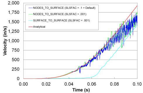
Figure 10. Velocity of the outside diameter of the journal bearing with various penalty stiffness scaling factors.
