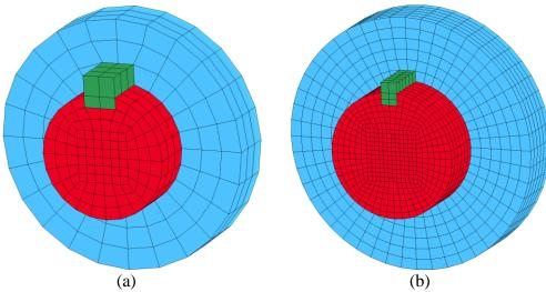
Figure 16. Finite element models with (a) a coarse mesh and (b) a refined mesh for the keyway test case.
