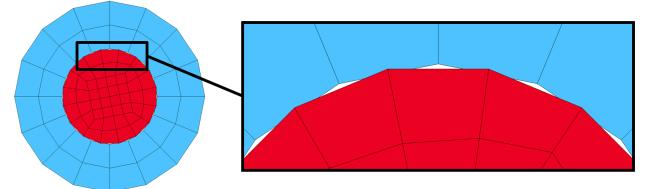
Figure 9. Incompatible mesh on the journal bearing and shaft can cause locking with NODE\_TO\_SURFACE contact.
