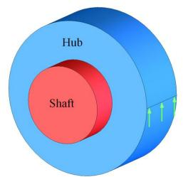
Figure 1. Example problem of an 8-inch diameter hub mounted on a 4-inch diameter shaft with a tangentially applied load.
