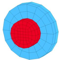
Figure 3. Mapped hexahedral mesh used in the journal bearing example problem.
