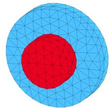
Figure 7. Tetrahedral mesh used in the journal bearing example problem.
