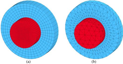
Figure 11. Refinements of (a) the hexahedral mesh and (b) the tetrahedral mesh.
