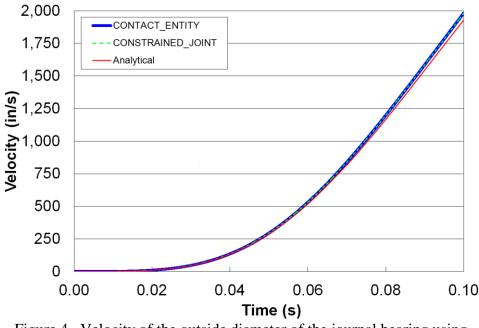
Figure 4. Velocity of the outside diameter of the journal bearing using \*CONTACT\_ENTITY and \*CONSTRAINED\_JOINT.
