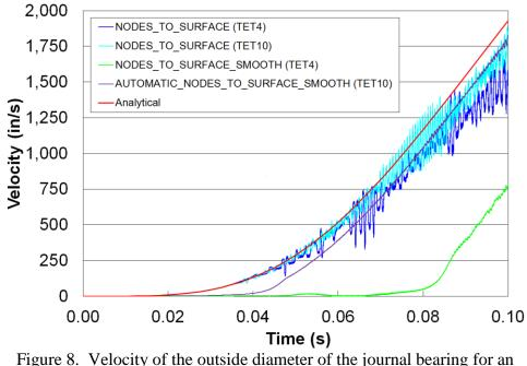
Figure 8. Velocity of the outside diameter of the journal bearing for a automatically generated tetrahedral mesh.
