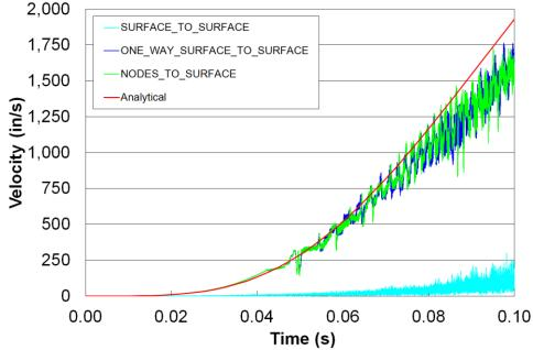
Figure 5. Velocity of the outside diameter of the journal bearing using three different penalty-based contacts.
