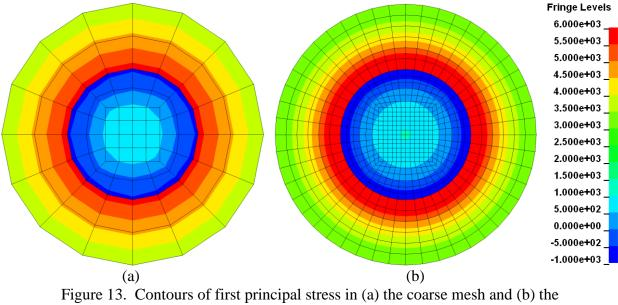
Figure 13. Contours of first principal stress in (a) the coarse mesh and (b) the refined mesh at the end of the dynamic relaxation phase using NODES\_TO\_SURFACE\_INTERFERENCE.
