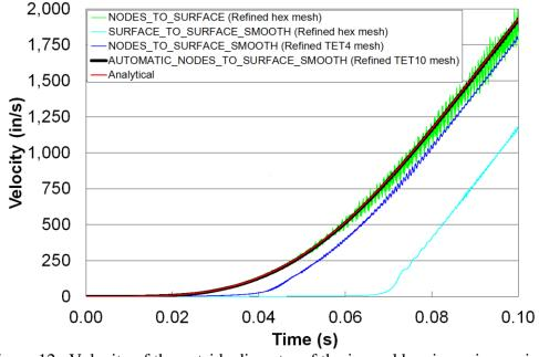
Figure 12. Velocity of the outside diameter of the journal bearing using various penalty-based contacts and refined element size.
