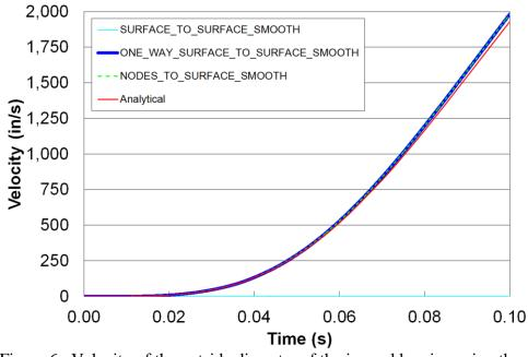
Figure 6. Velocity of the outside diameter of the journal bearing using three different penalty-based smooth contacts.
