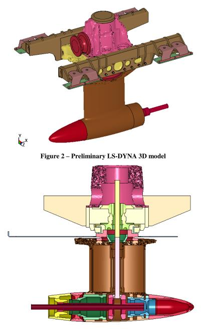
Figure 3 – Preliminary LS-DYNA 3D model – Internal transmission system elements
