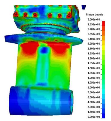
Figure 10 - 3D LS-DYNA simulation results - Von Mises stress results on POD principal parts
