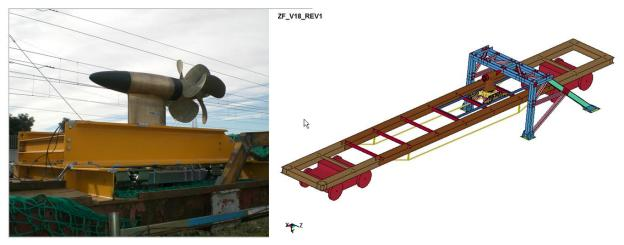
Figure 7 – Experimental set up and detailed numerical model
