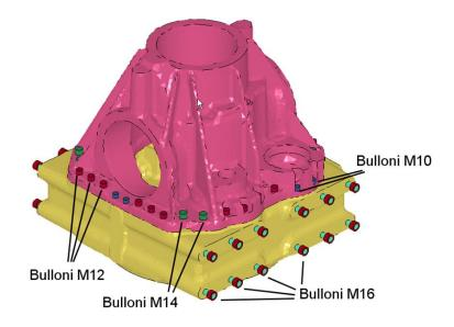
**Figure 6 – Connection bolts models**
