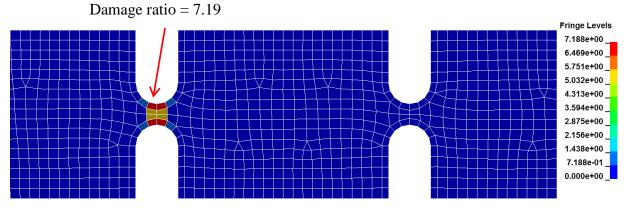
Figure 12 - Cumulative damage ratio by Steinberg's method
