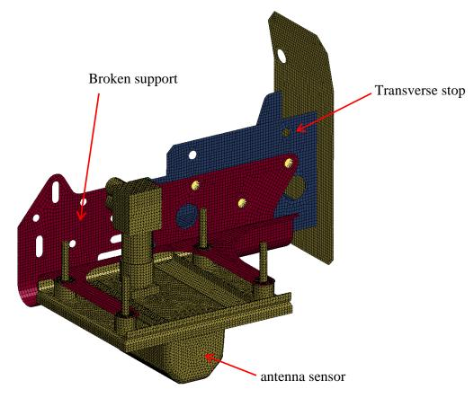
Figure 14 (a) – global view of support antenna model
