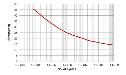
Figure 2 – S-N fatigue curve
