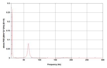
Figure 10 – Stress PSD at critical point
