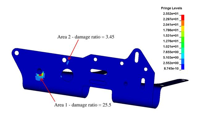
Figure 16 (a) – cumulative damage according Steinberg's method
