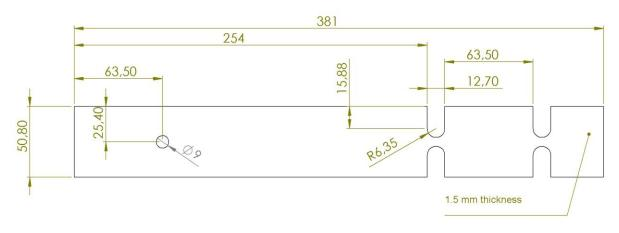
Figure 5 – aluminum beam using for the shaker table experiment (all dimensions are in millimeter)
