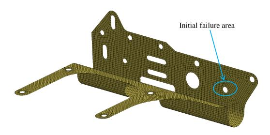
Figure 15 – broken support
