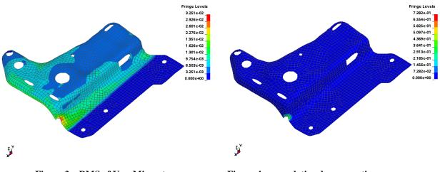
Figure 3 – RMS of Von-Mises stress
