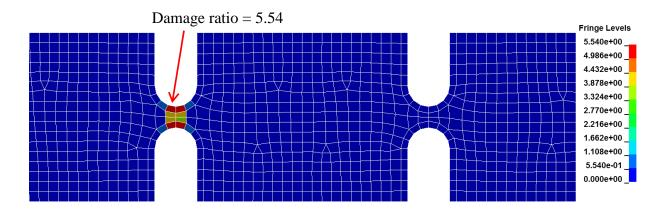
Figure 11 - Cumulative damage ratio by Dirlik method
