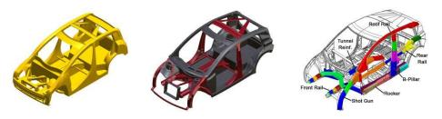
Figure 13: LF3G optimization, reference body structure and structural sub-systems
