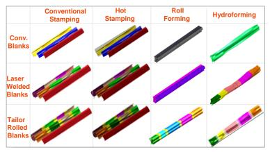
Figure 14: Rocker Solution Alternative Manufacturing Scenarios
