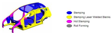
Figure 16: FSV body-in-white manufacturing processes
