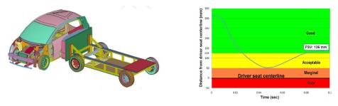
Figure 19: IIHS side impact crash test and B-pillar intrusion
