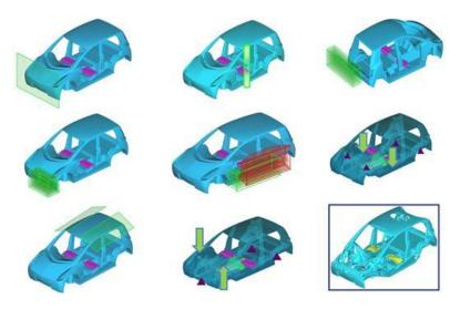
Figure 5: ACP Process MD Topology Optimization for the Vehicle Skeleton (FSV)
