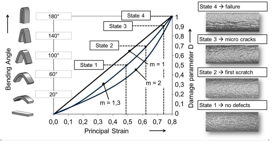
$\rightarrow$  Calibration of damage model GISSMO
