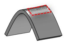
Pre-stage of bending process  $\rightarrow$  no damage
