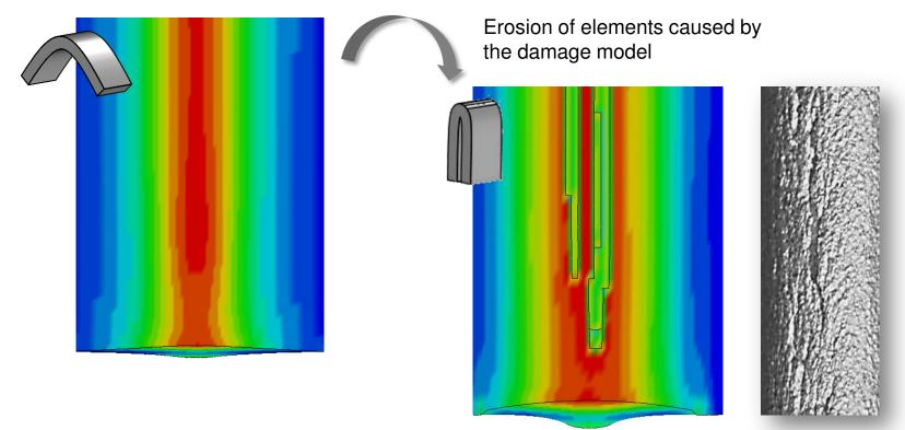
→ Good correlation between real surface defect and calculated damage value
