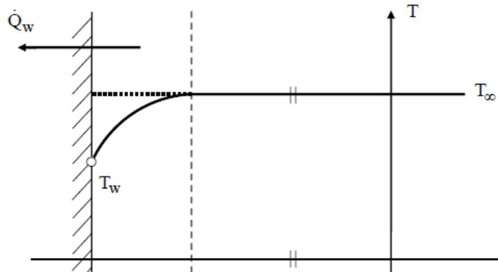
Fig.10: temperature distribution in the fluid near a solid wall
