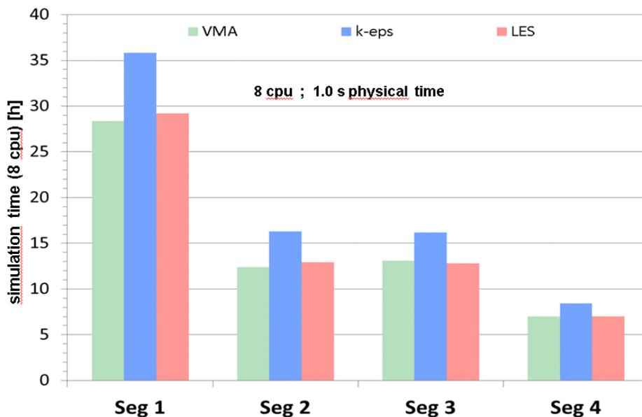
Fig.6: simulations with different turbulence models; comparison of runtimes (same mesh size)
