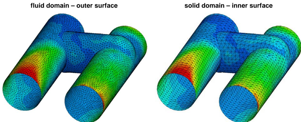
Fig.8: coupling: mesh and temperature distribution on the common boundary
