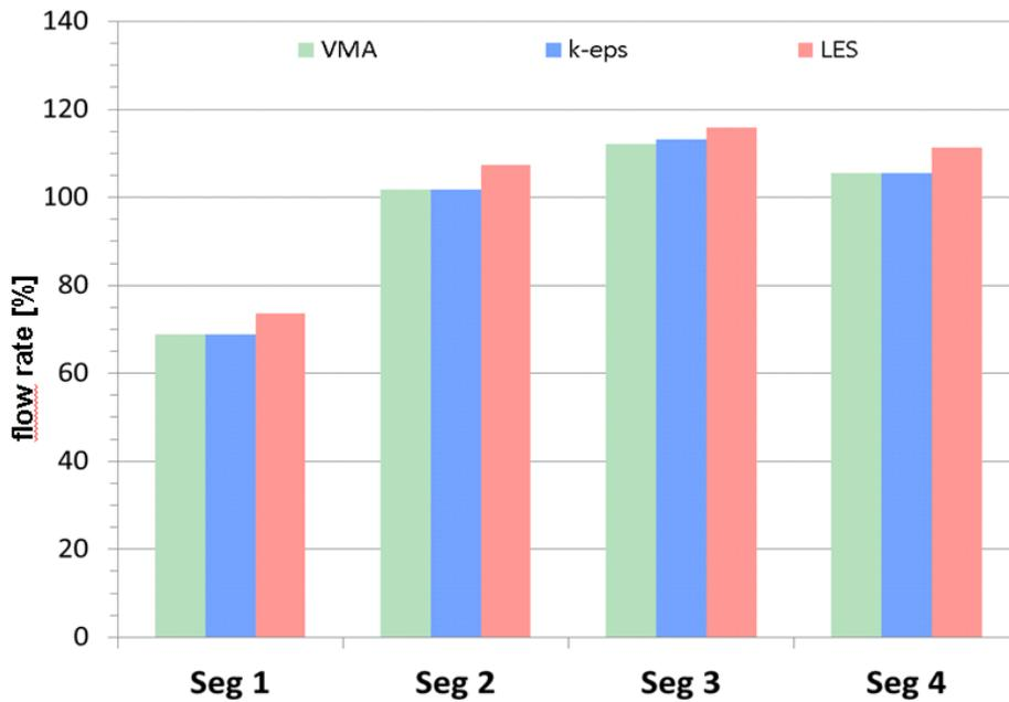
Fig.5: simulations with different turbulence models; comparison of flow rate (all segments)
