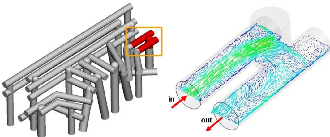
Fig.3: u-bend section of punch segment 1 (left) and vector plot of velocity (right)
