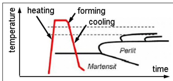
Fig.1: typical temperature profile of press hardening process in TTT diagram
