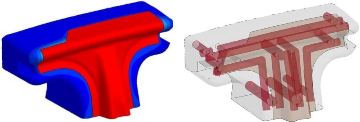
Fig.7: punch segment 4 with blank (red); left image shows a fringe plot of temperature at time  $t=0$ ; right image shows the geometry of tool and blank in transparent mode
