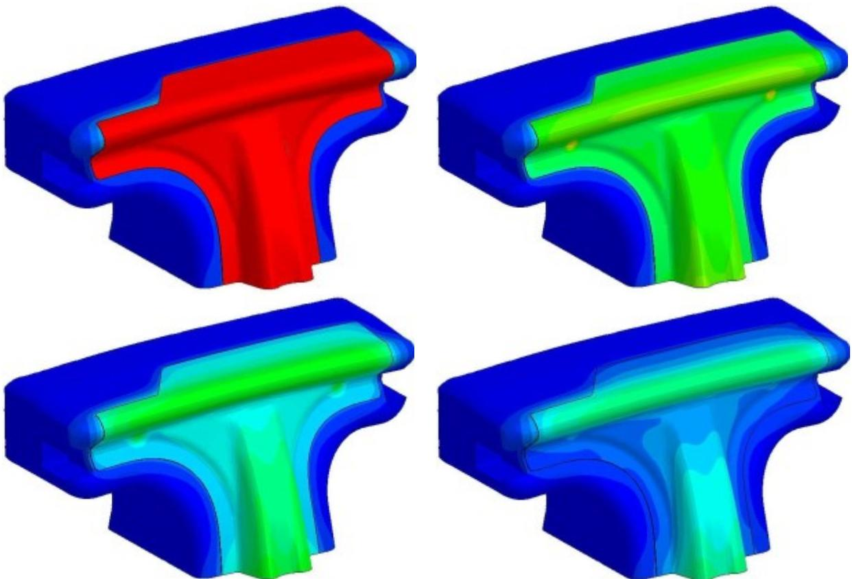
Fig.11: fringe plot of temperature in tool and blank during one cycle
