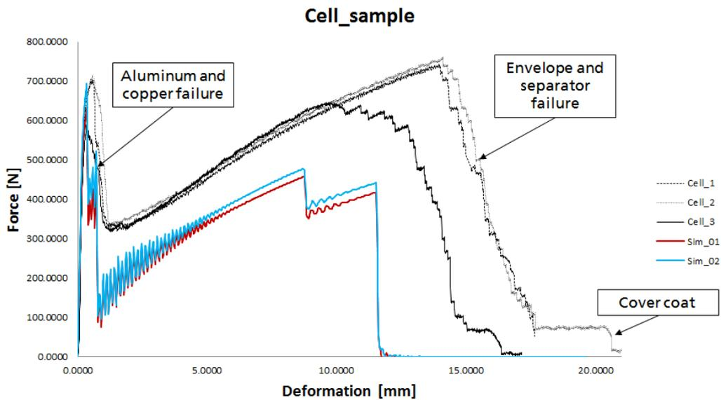
Fig.13: Validation of the cell model.
