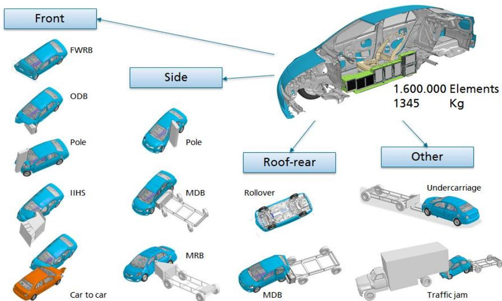
Fig.8: Crash simulations performed in the EVERS SAFE project.
