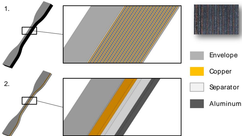
Fig.12: Numerical Model of Battery Cell (1-Detailed, 2-Simplified).
