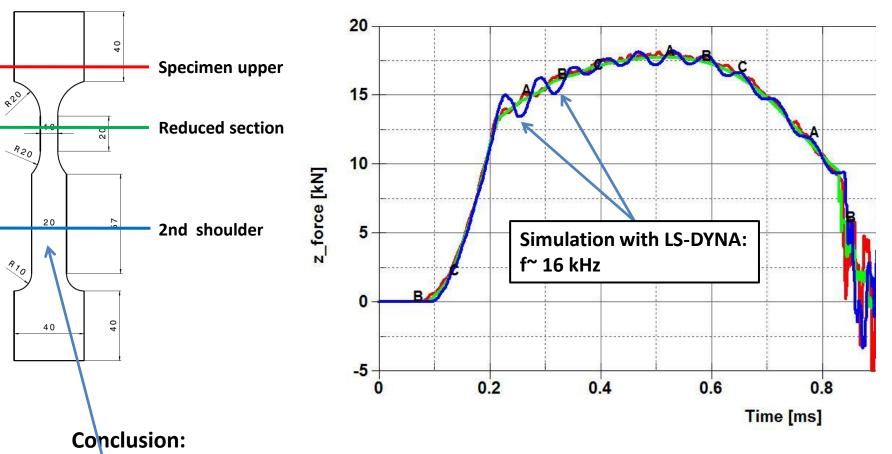
**1.** negletible oscillation within the reduced section of the specimen
