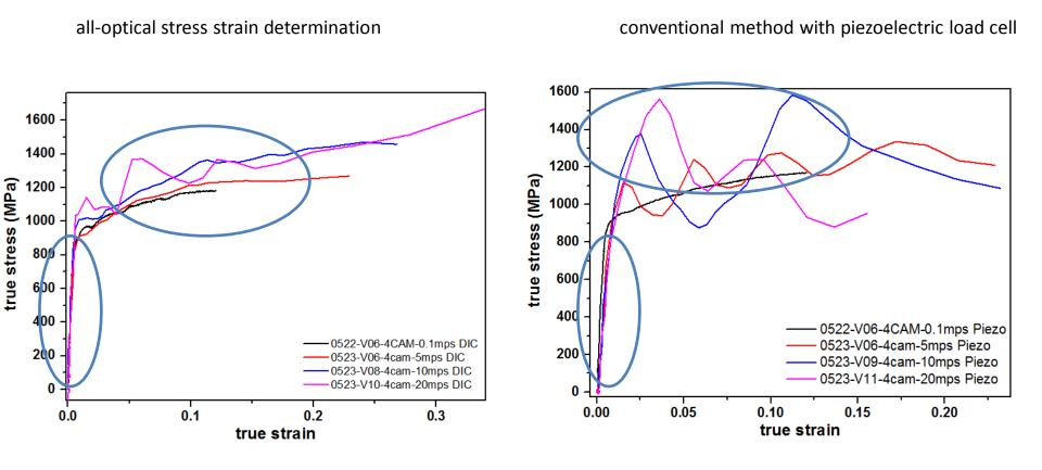
conclusion: negligible oscillation up to 10 m/s much lower oscillation at 20 m/s -> can be further reduced with better specimen geometry and changes on test equipment!
