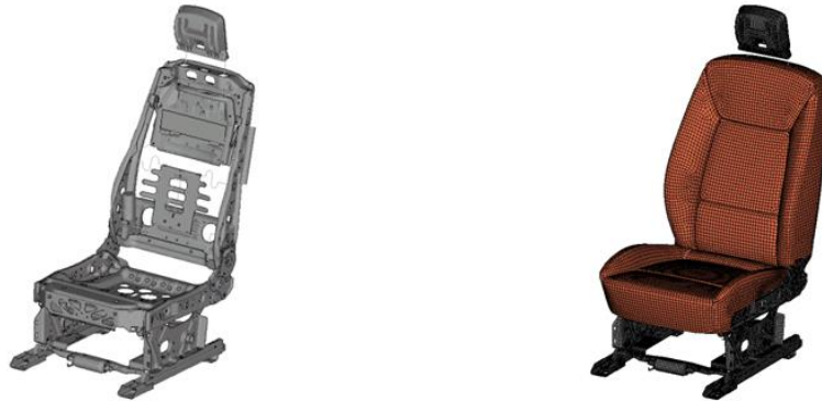
Fig.1: Finite-Element-Model of Seat Structure and Unoccupied Seat (courtesy of Ford).
