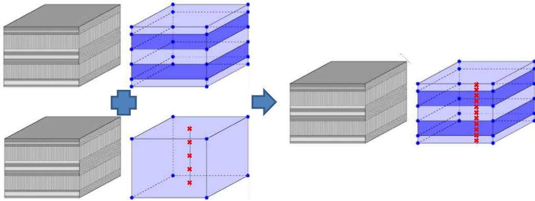
Fig.5: Combined stacked and layered t-shell approach on the basis of [9]
