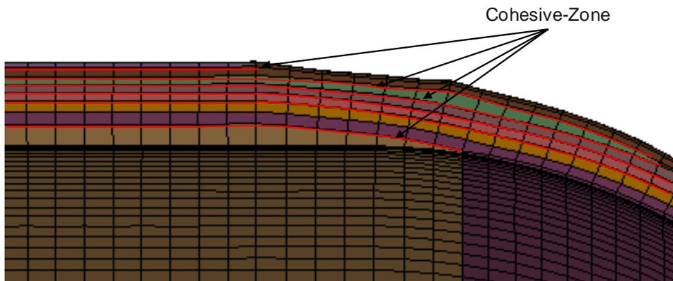
Fig.2: Sectional view of the mesh of the winding structure
