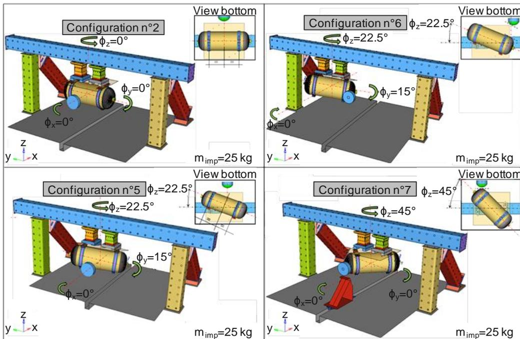
Fig.19: Impact configurations for test programme
