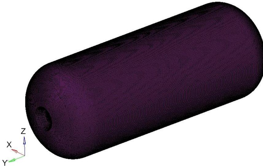
Fig.3: Mesh of liner
