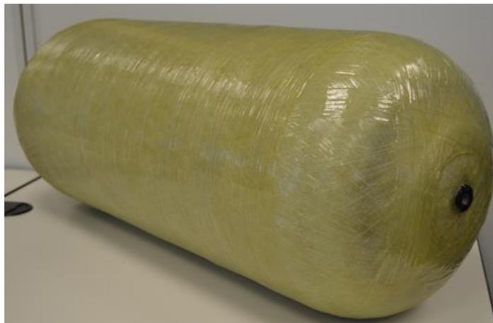
Fig.1: Type IV CNG tank
