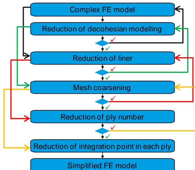
Fig.21: Iterative simplification process
