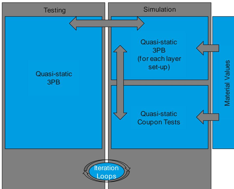
Fig.9: Material validation process for thick UD structures of MATISSE
