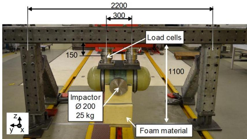
Fig.18: Test rig for impact tests on tank level
