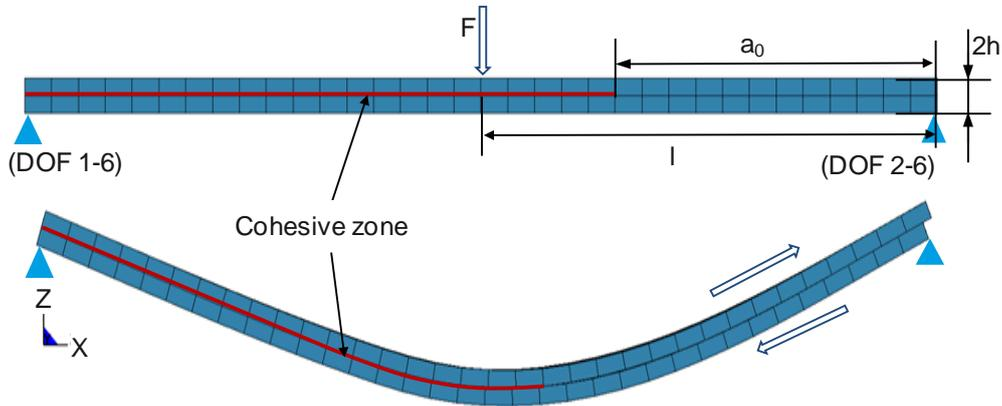
Fig.15: FE model of ENF test specimen in undeformed (top) and deformed (bottom) shape
