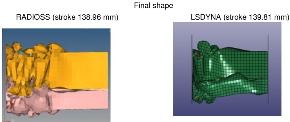
Fig.16: RADIOSS final shape of crushed beam
