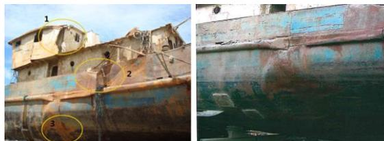
Fig. 6: Collision damage configuration of struck ship
