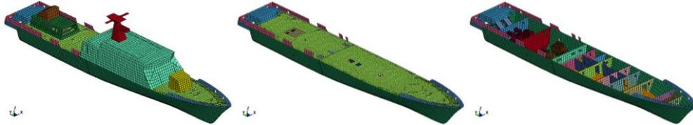
Fig. 21: F.E. mesh configuration of ship including openings on deck and superstructure, and watertight bulkheads
