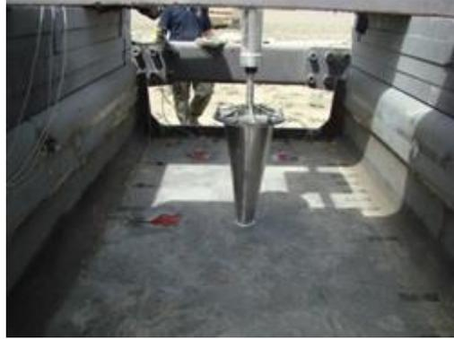
Fig. 15: Deformation cone used for total deformation measurement.
