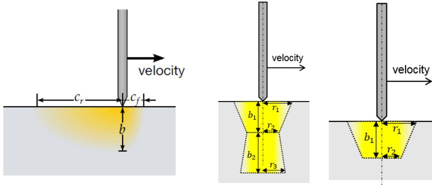
Fig.3: Ellipsoid heat source (left), double conical heat source (middle), conical heat source (right)
