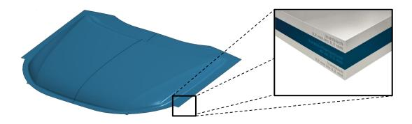
Modelling with one layer of shells obviously not sufficient!
