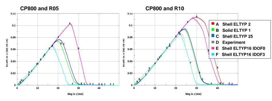
Failure data has been calibrated for plane stress states using DIEM, TYP=1 shear failure model:
