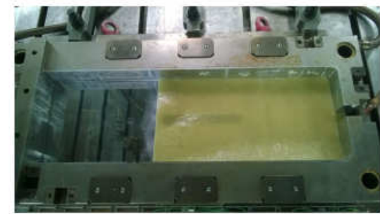
Mould charged with approx. 60% of semi-finished product
