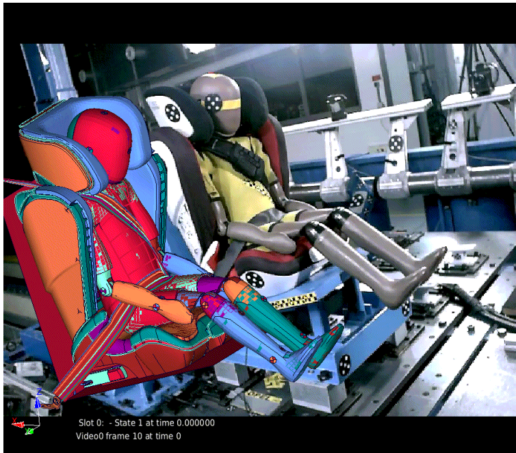
Rigid fixture test with generic pulse: Dummy: Humanetics_Q6_V2.0.3_S3 CRS: Römer Kidfix XP
