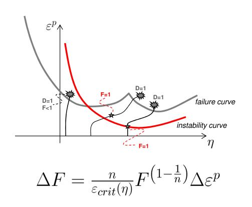
Similar to damage, an instability measure is incrementally accumulated as a function of the plastic strain increment and of the failure curve. **Coupling begins when F = 1!**  DCRIT assumes the value of current damage when coupling begins.
