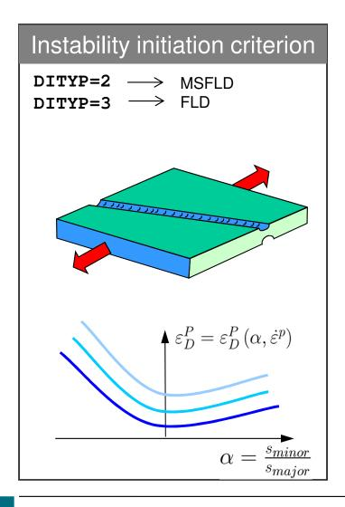
The MSFLD damage initiation criterion (DITYP=2) only considers the evolution of plastic strain if the pressure is negative (i.e., compressive stress states have no effect). The damage initiation variable is defined as
