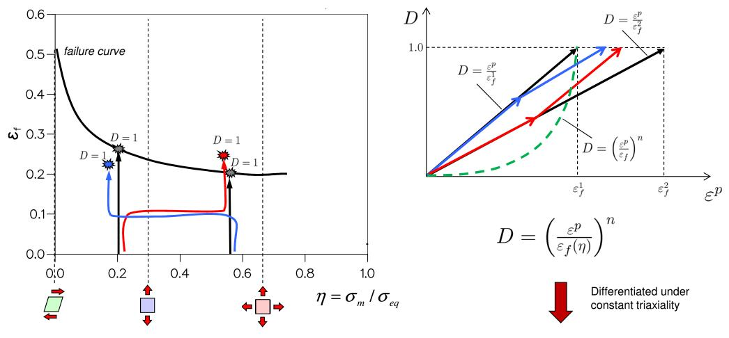
Damage is incrementally accumulated as a function of the plastic strain increment and of the failure curve. **Failure occurs when D = 1!**
