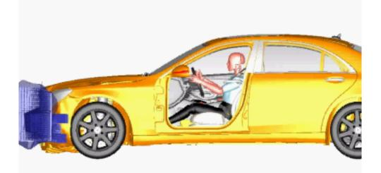
II: Model reduction to occupant cell (sled) model with vehicle movement
