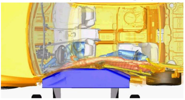
• Focus on analyzing the crash interaction and design setup of side airbag systems, door trim (arm rest, pelvis support), seat assembly (esp. backrest), side trims and belt tensioning
