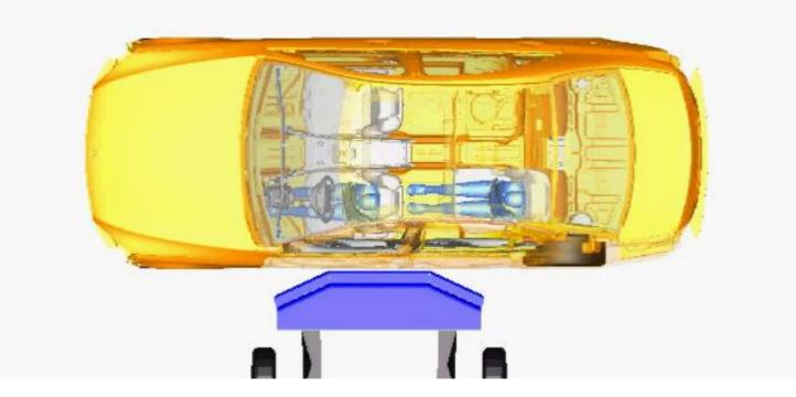
• All occupant simulations are running completely integrated into the structure model (no subsystem)
