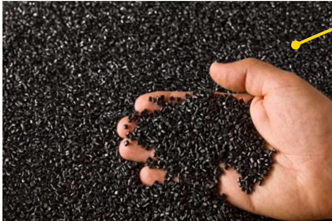
Short-Fiber-Reinforced Plastic Resin (fiber length: ~ 0,1 - 0,5 mm)
