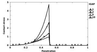
Contact is released if penetration is larger than half characteristic length after equilibrium
