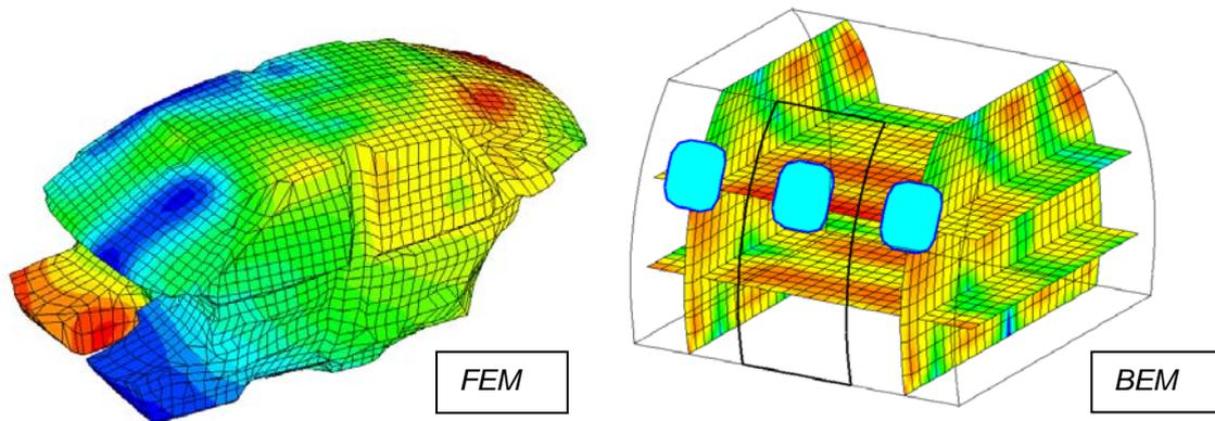
Figure 1: Sound pressure in a car and in a cabin section of an aircraft
