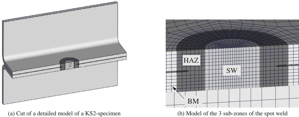
Figure 3: Detailed Model of Spot Weld
