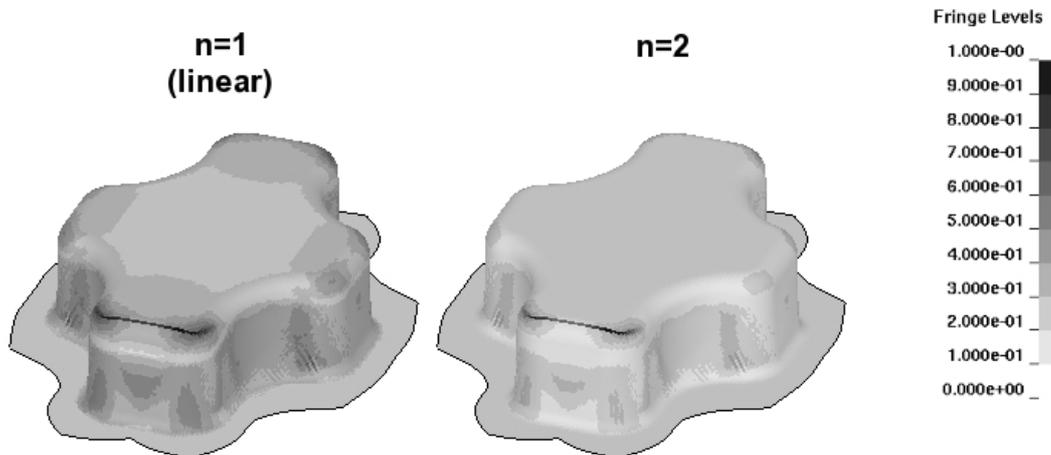
Figure 7: Cross-die; contours of damage  $D$
