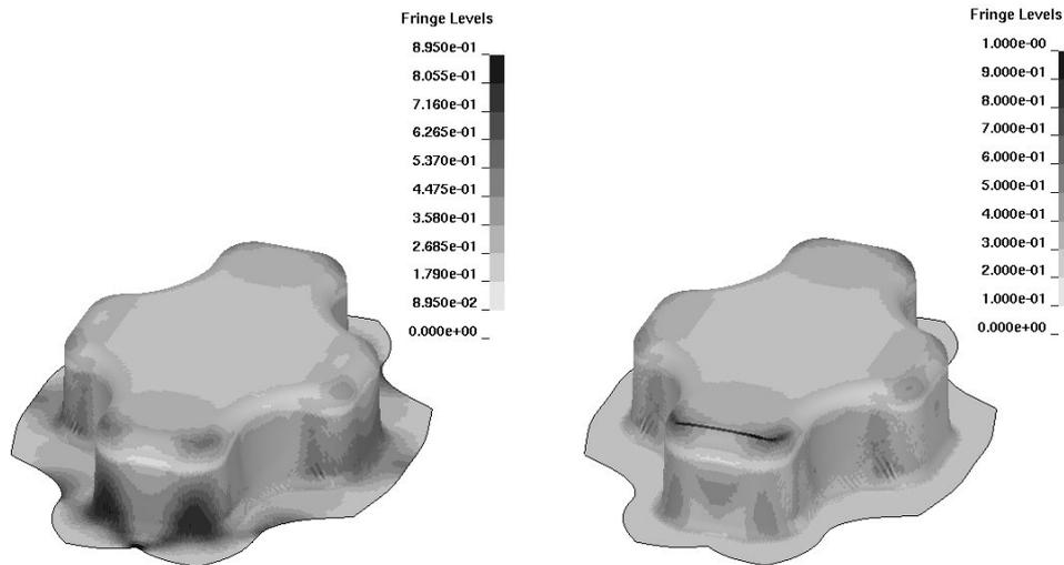
Figure 6: Cross-die; Contours of equivalent plastic strain (left) and damage  $D$  (right)
