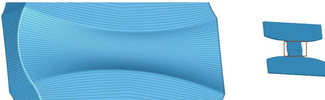
Figure 4: Finite element discretization of butterfly specimen at the critical location (centre)
