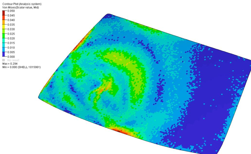
Figure 4: Simple elasto-plastic model with regular quad mesh
