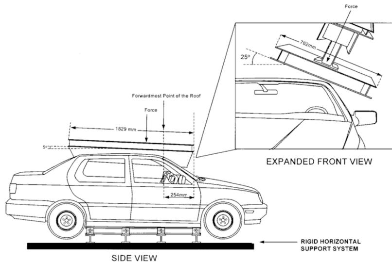
Figure 13: roof crush load case
