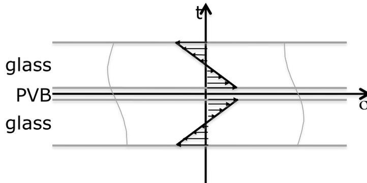
Figure 15: pre-stresses in laminated glass because of production process
