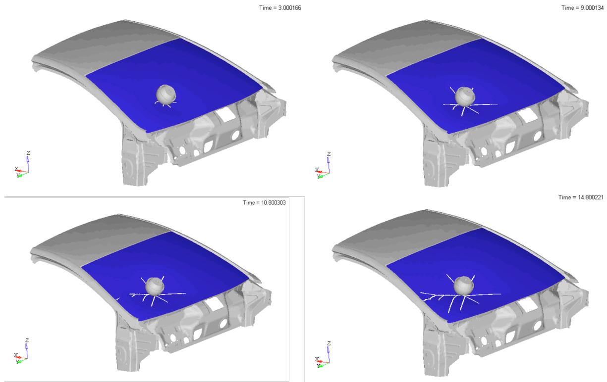
Figure 10: Windscreen circular tria mesh (around impact point)
