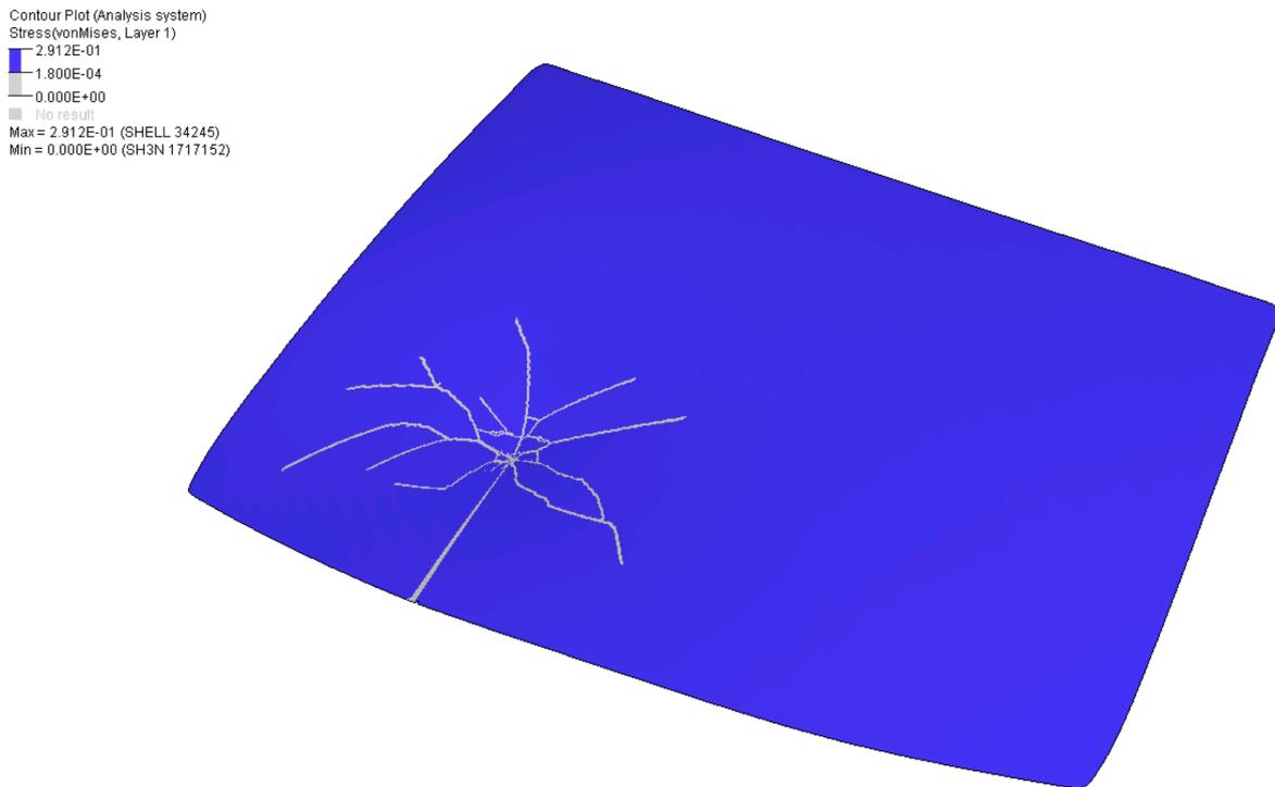
Figure 6: Improved laminated glass model respecting rupture with regular tria mesh
