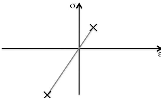
Figure 16: different glass rupture stress in traction and compression direction
