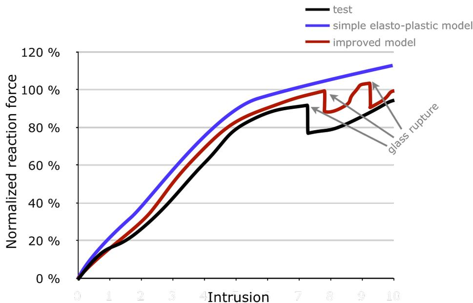
Figure 14: roof crush – normalized reaction force over intrusion
