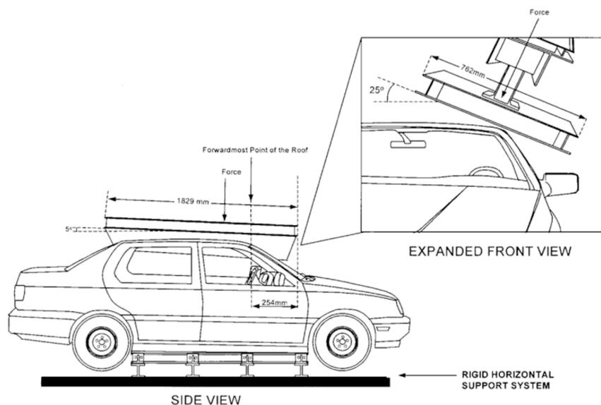
Figure 2: roof crush
