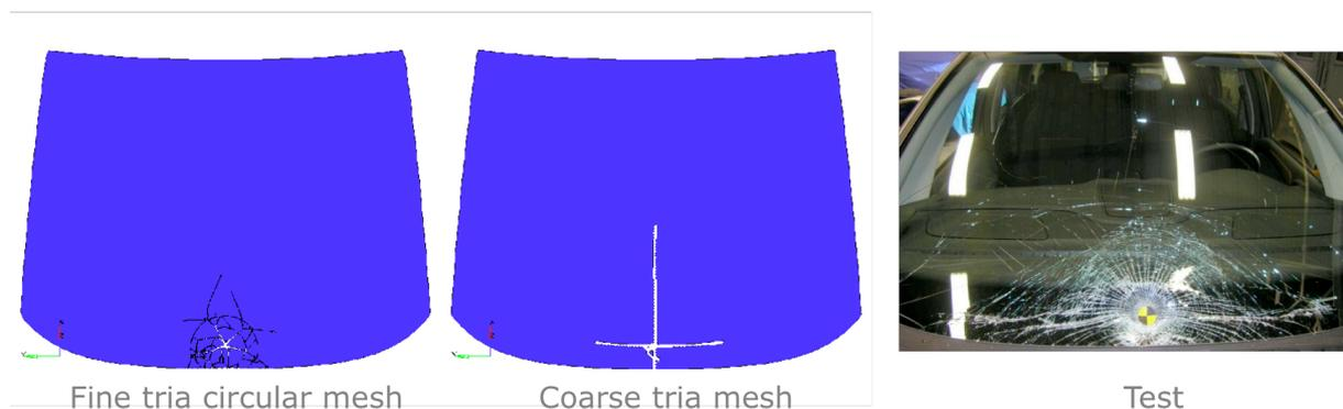
Figure 12: rupture behaviour (impact in cowl area)
