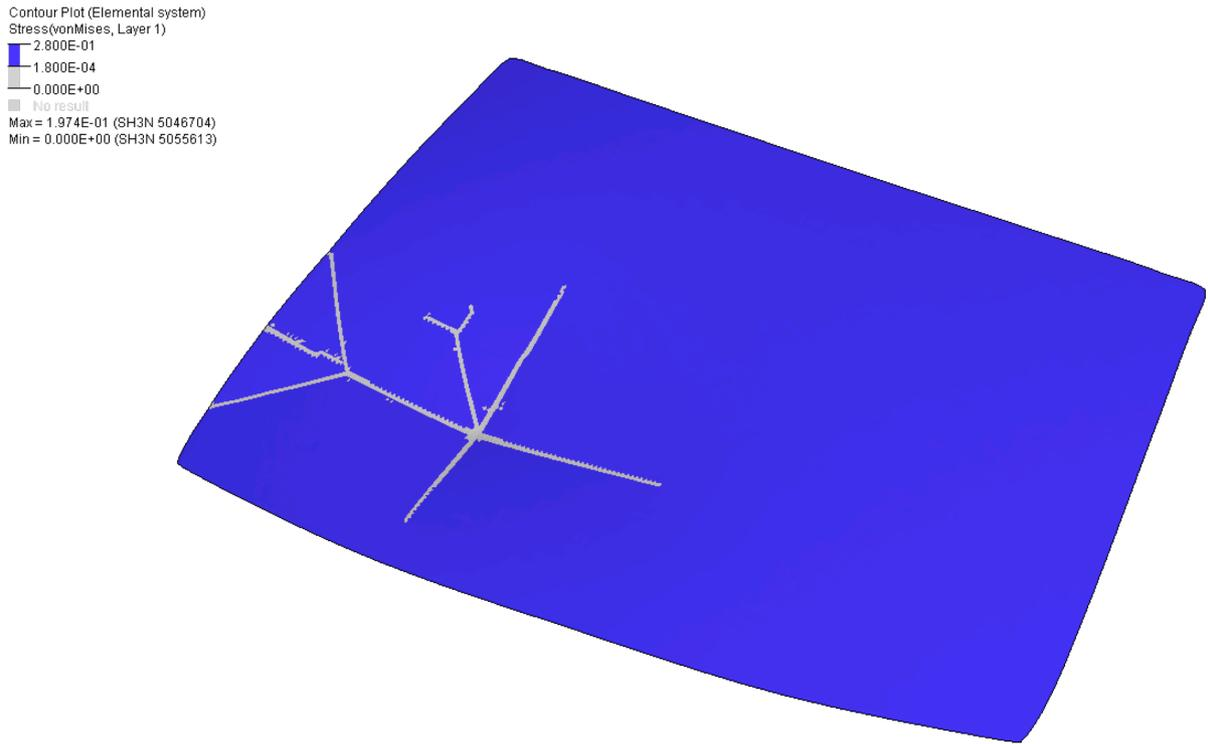
Figure 5: Improved laminated glass model respecting rupture with regular tria mesh
