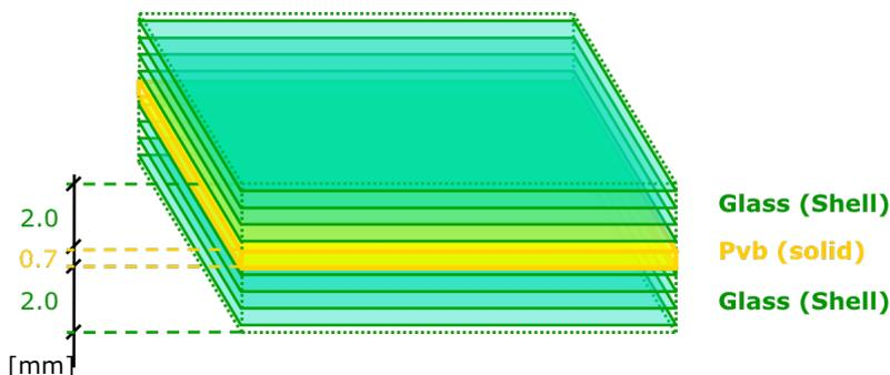
Figure 17: next step: shell-solid-shell model
