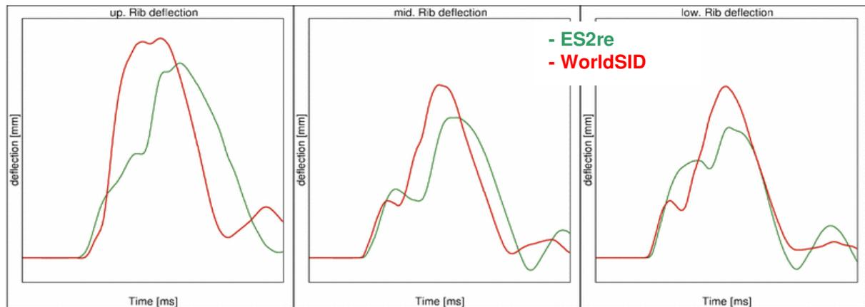
Figure 26: vehicle oblique pole; Upper, middle and lower thorax rib deflections [mm] vs. Time [ms].
