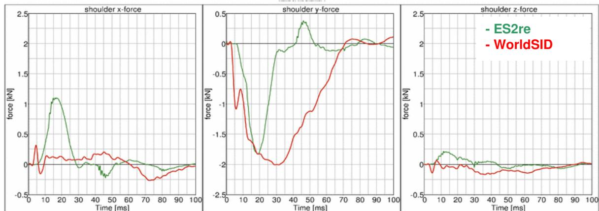
Figure 20: flat barrier 4 m/s; Shoulder force [kN] in x-, y- and z-direction vs. Time [ms].
