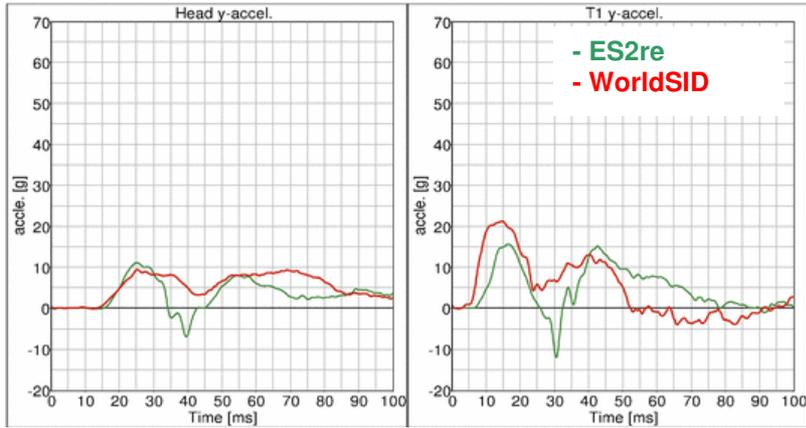
Figure 16: flat barrier 4 m/s; Head and T1 y-acceleration [g] vs. Time [ms].
