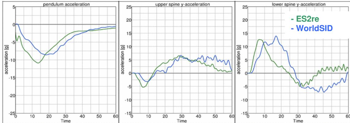
Figure 6: 3.0 m/s abdomen test; Pendulum, lower spine and upper spine acceleration [g] vs. Time [ms].
