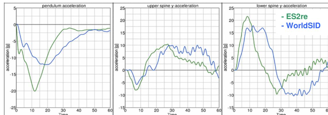
Figure 8: 4.3 m/s abdomen test; Pendulum, lower spine and upper spine acceleration [g] vs. Time [ms].
