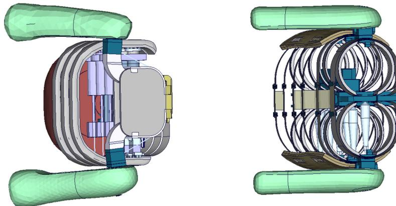
Below the clavicle/shoulder rib, both dummies consist of three thorax ribs. On the ES2re ribs a CONFOR® pink foam is tied on each single rib. The WorldSID ribs are covered with an ensolite foam pad which is only connected by a hook-and-loop fastener.
