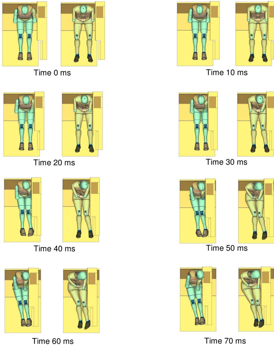
Figure 21: flat barrier 4 m/s; left hand side ES2re, right hand side WorldSID for times 0 - 70 ms
