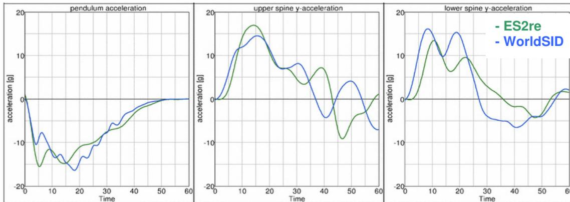
Figure 3: 4.3 m/s thorax test; pendulum, upper spine and lower spine accelerations [g] vs. time [ms].
