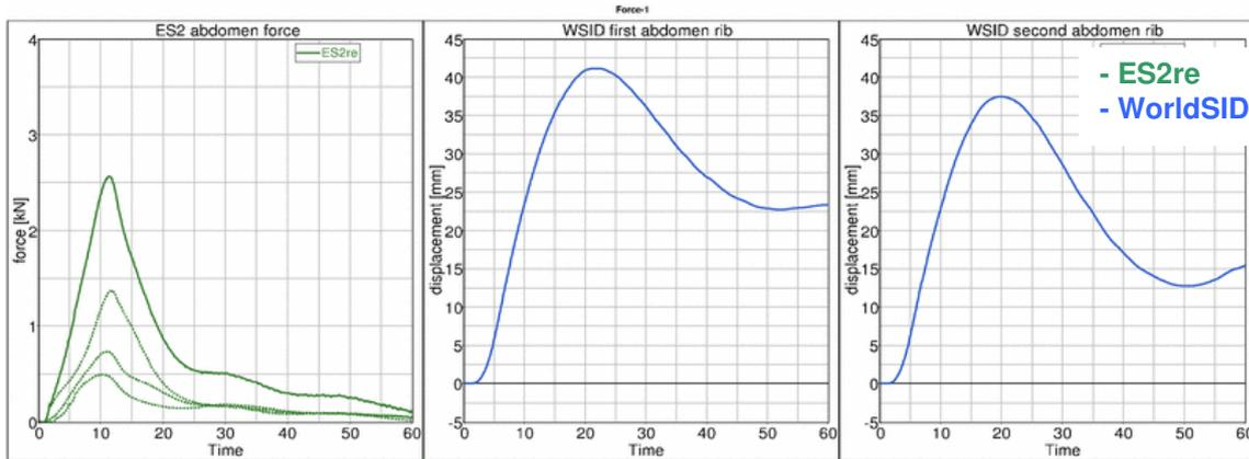
Figure 9: 4.3 m/s abdomen test; ES2re abdomen forces [kN] and WorldSID upper and lower abdomen rib deflection [mm] vs. Time [ms]
