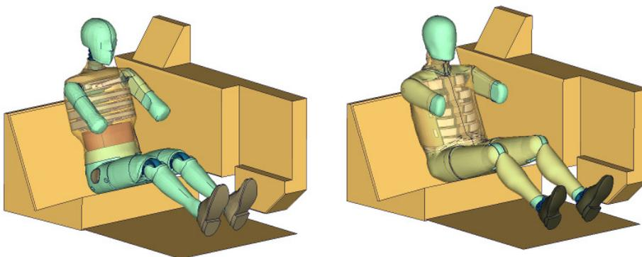
Figure 15: ES2re (left hand side) and WorldSID (right hand side) sled test with flat barrier and 4 m/s.
