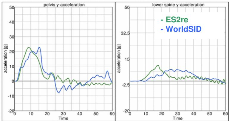
Figure 11: 4.0 m/s pelvis test; pelvis and lower spine acceleration [g] vs. Time [ms].
