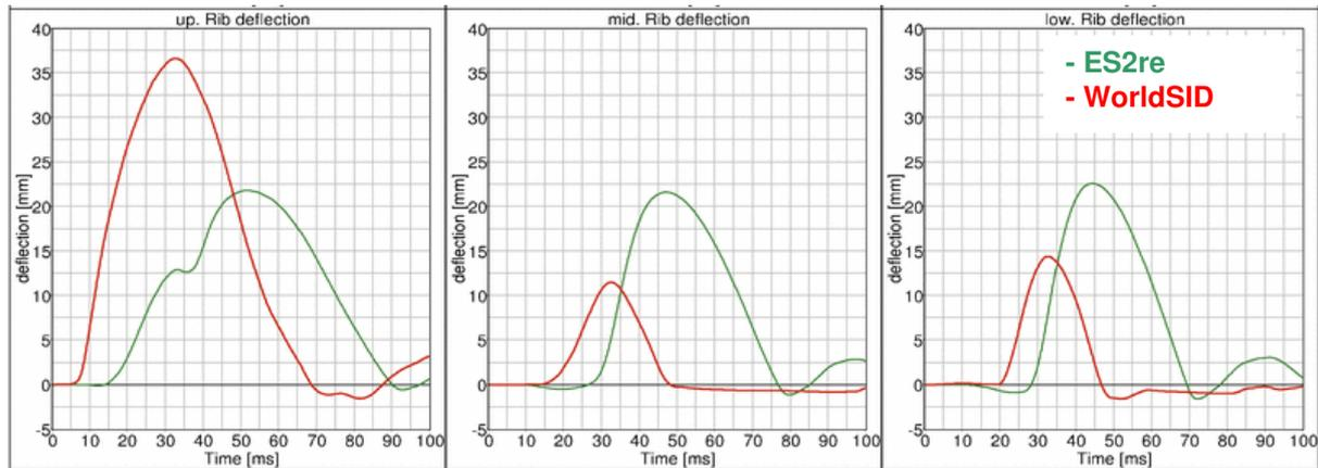
Figure 18: flat barrier 4 m/s; Upper, middle and lower thorax rib deflections [mm] vs. Time [ms].
