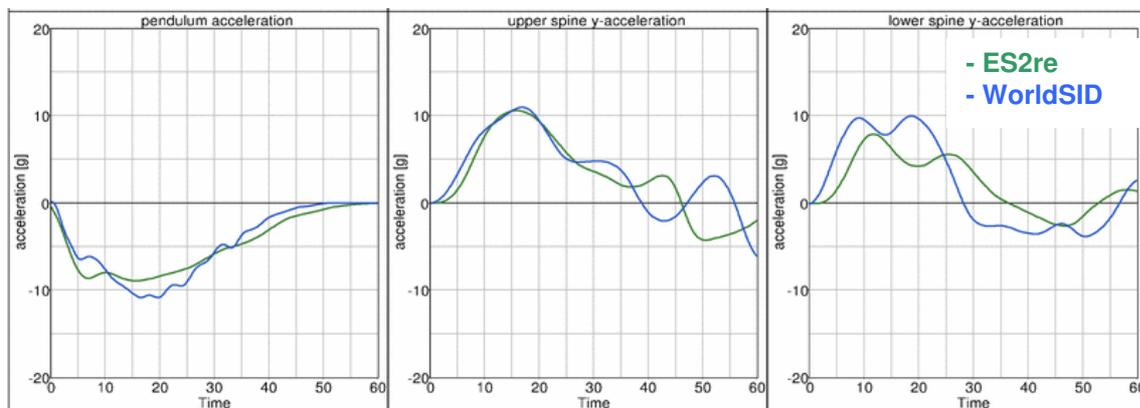
Figure 1: 3.0 m/s thorax test; pendulum, upper spine and lower spine accelerations [g] vs. time [ms].
