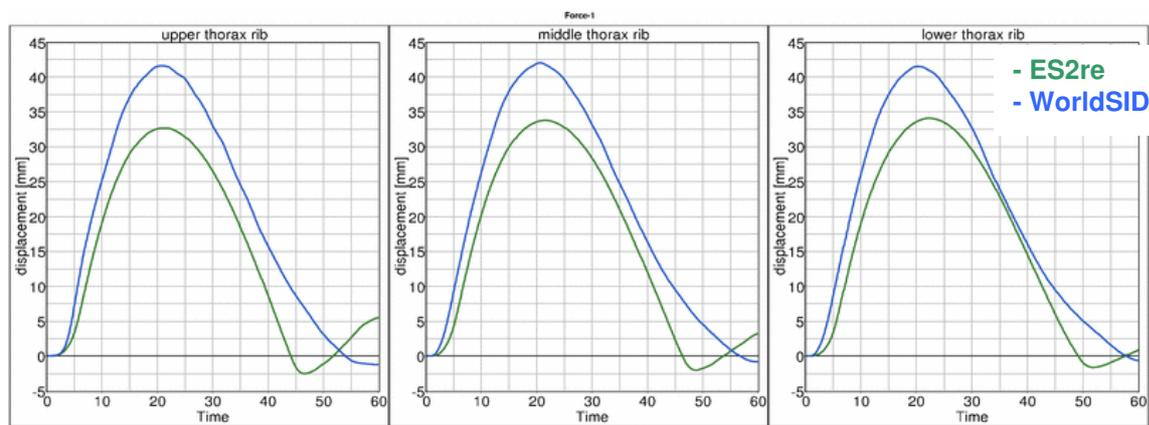
Figure 4: 4.3 m/s thorax test; upper, middle and lower thorax rib deflection [mm] vs. time [ms].
