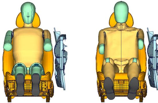
Figure 22: ES2re (left hand side) and WorldSID (right hand side) in vehicle with door trim and seat front view.
