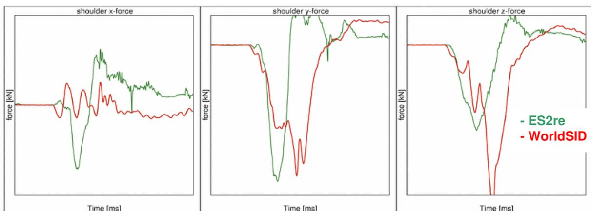
Figure 25: vehicle oblique pole; Shoulder force [kN] in x-, y- and z-direction vs. Time [ms].
