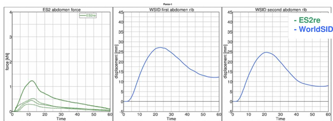
Figure 7: 3.0 m/s abdomen test; ES2re abdomen forces [kN] and WorldSID upper and lower abdomen rib deflection [mm] vs. Time [ms]
