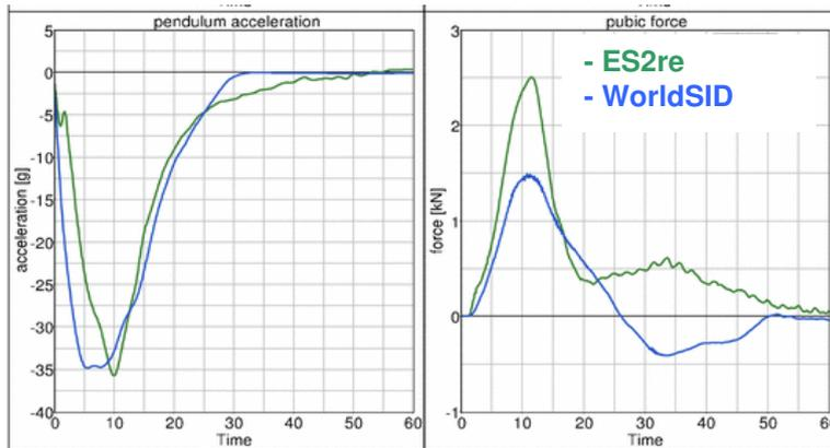
Figure 14: 6.7 m/s pelvis test; Pendulum acceleration [g] and pubic force [kN] vs. Time [ms].
