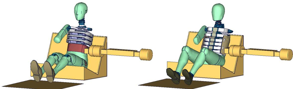
Figure 5: ES2re abdomen pendulum test (left hand side) and WorldSID abdomen pendulum test (right hand side)
