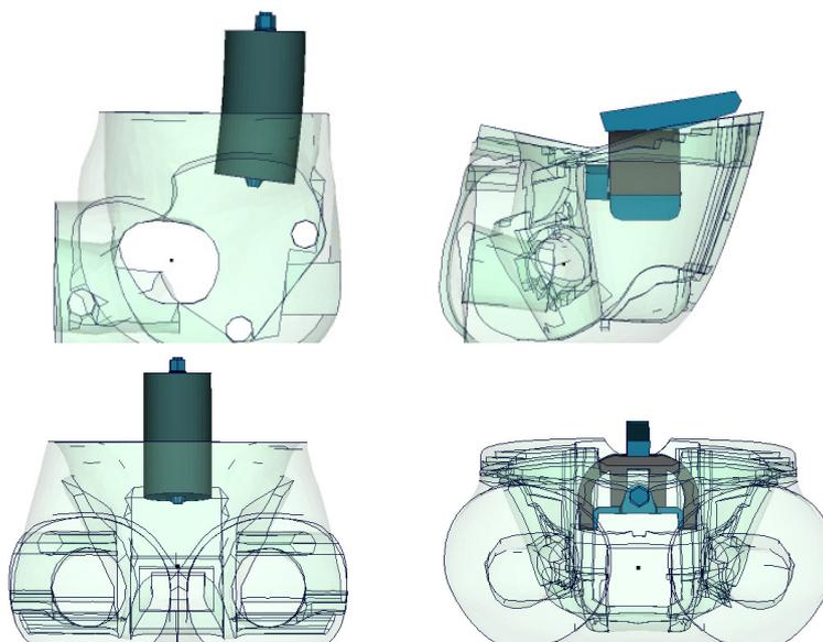
Figure 6: lumbar spine of ES2re (left hand side) and WorldSID (right hand side) in side view and front view.
