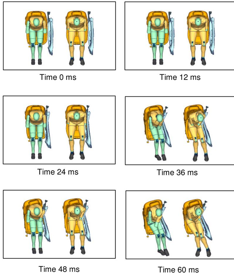
Figure 24: vehicle oblique pole; left hand side ES2re, right hand side WorldSID for times 0 - 60 ms
