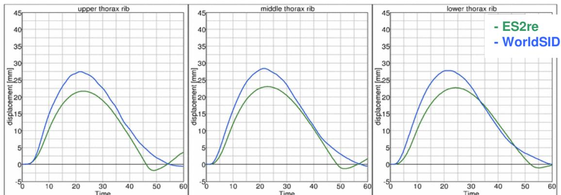
Figure 2: 3.0 m/s thorax test; upper, middle and lower thorax rib deflection [mm] vs. time [ms].
