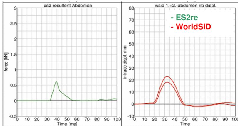
Figure 19: flat barrier 4 m/s; ES2re resultant abdomen force [kN] and WorldSID abdomen rib deflections [mm] vs. Time [ms].
