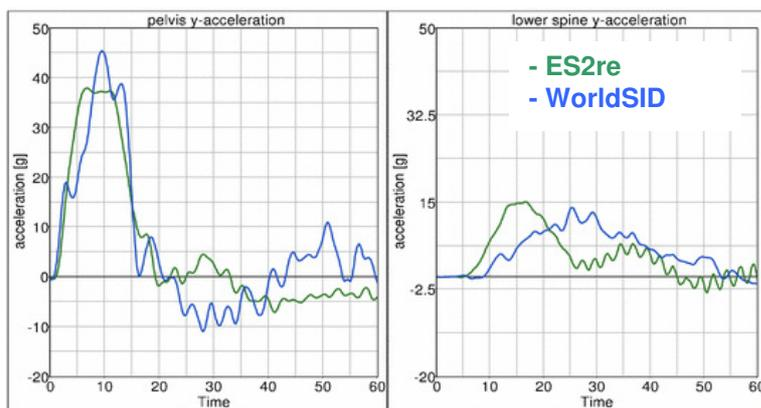
Figure 13: 6.7 m/s pelvis test; Pelvis and lower spine acceleration [g] vs. Time [ms].
