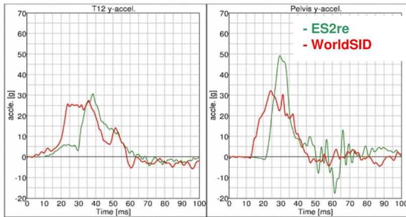
Figure 17: flat barrier 4 m/s; T12 and pelvis y-acceleration [g] vs. Time [ms].
