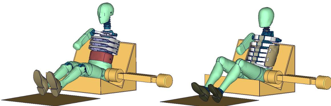
Figure 10: ES2re pelvis pendulum test (left hand side) and WorldSID pelvis pendulum test (right hand side)
