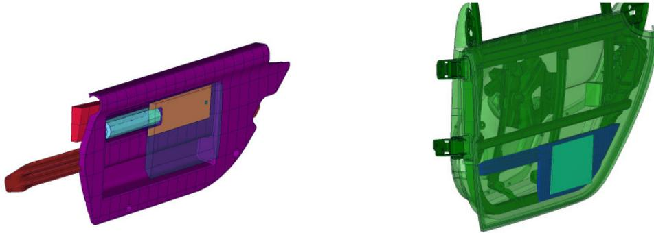
Fig 2: The Active Door Module and the Active Door Module mounted in the door.
