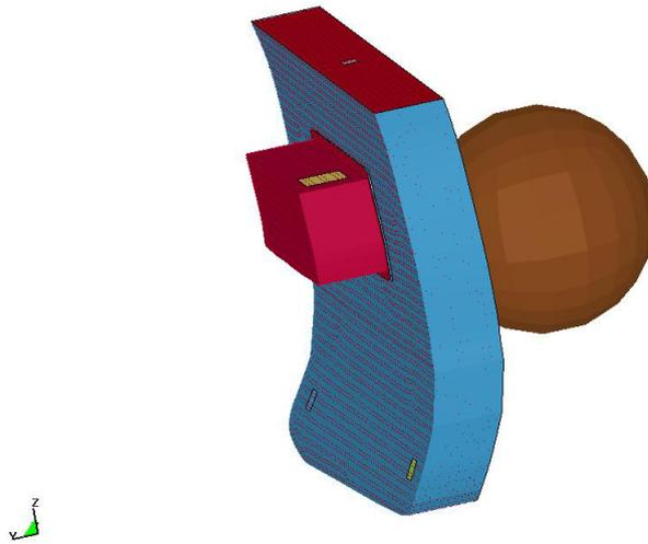
Fig.5: Rigid Ball Impact onto a Side Door
