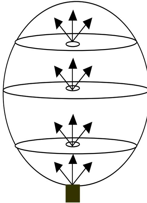
Fig.8: Multiple Chambered Airbag
