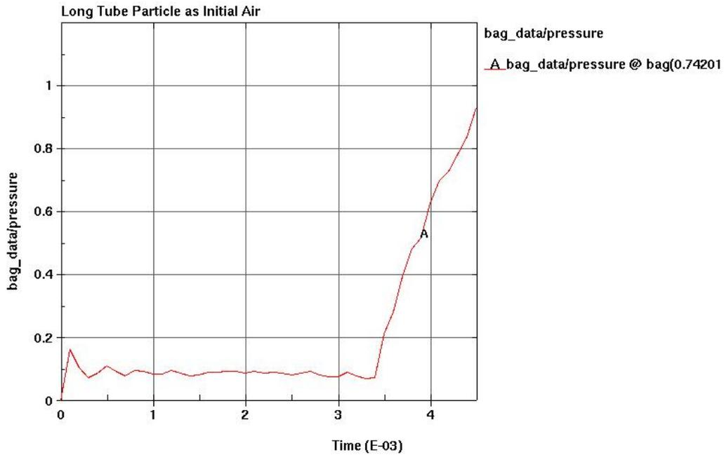
Fig.3: Pressure Time Histories for Particle Method
