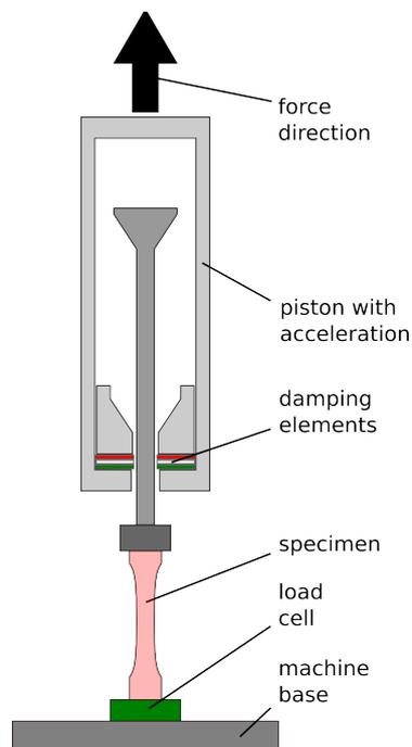
Figure 2: Schematic setup of the servo-hydraulic testing machine
