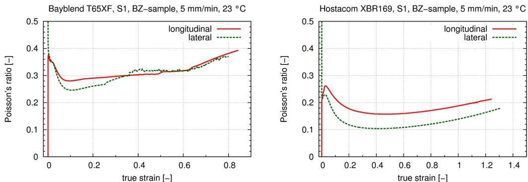
Figure 7: Poisson's ratio for Bayblend T65XF (left) and Hostacom XBR169G S1 (left)
