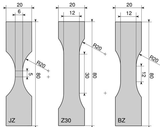
Figure 3: Different sample geometries for the tensile test
