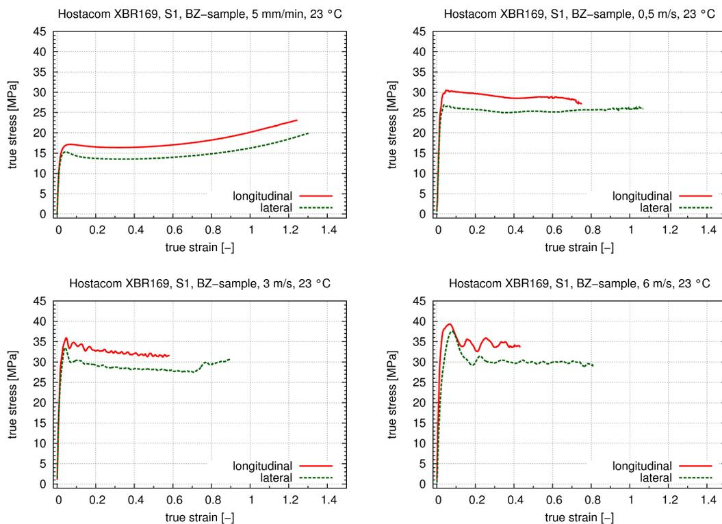
Figure 11: Stress-strain-behaviour for Hostacom XBR169G at setting S1 at various strain rates
