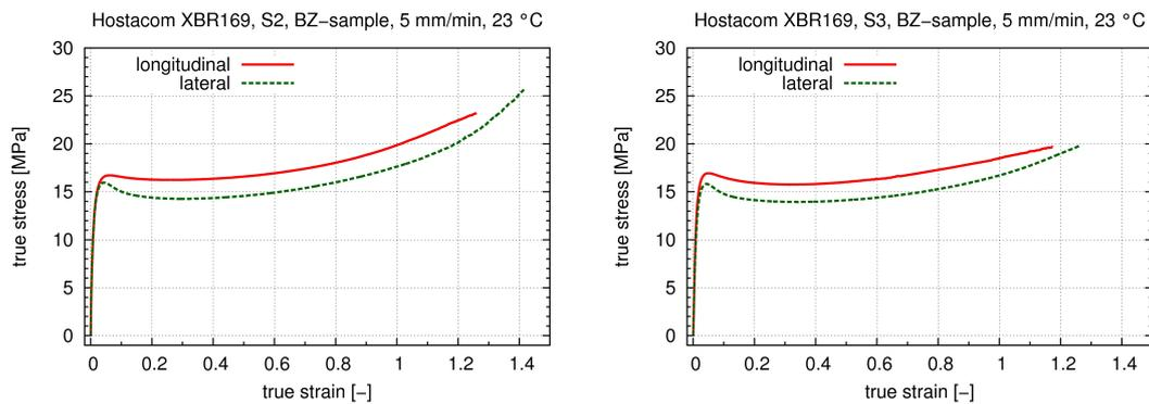
Figure 9: Stress-strain-behaviour for Hostacom XBR169G; left: setting S2; right: setting S3
