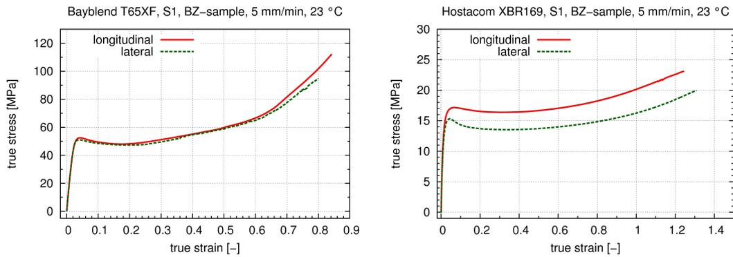
Figure 6: Stress-strain-behaviour; left: Bayblend T65XF; right: Hostacom XBR169G
