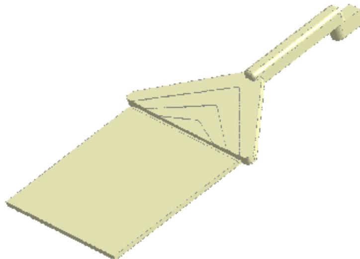
Figure 1: Injection moulded plate with delta gate
