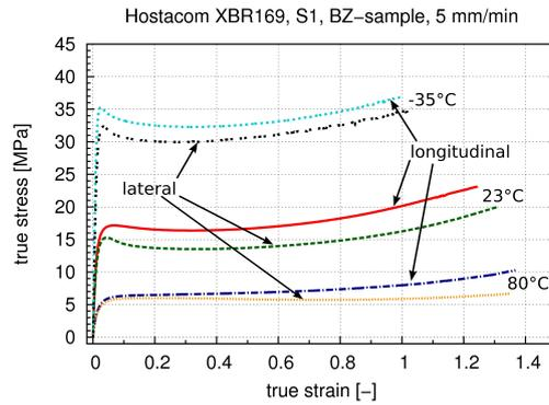
Figure 10: Influence of testing temperature for Hostacom XBR169G at setting S1
