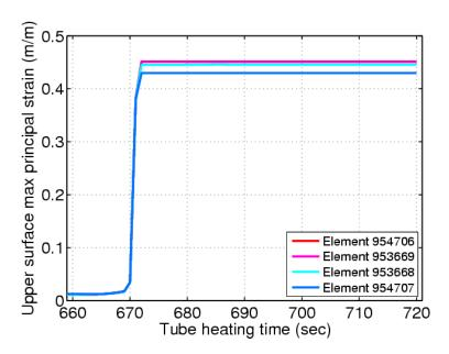
Figure 9: Evolution of the upper surface maximum principal strain of four elements as pressure increases
