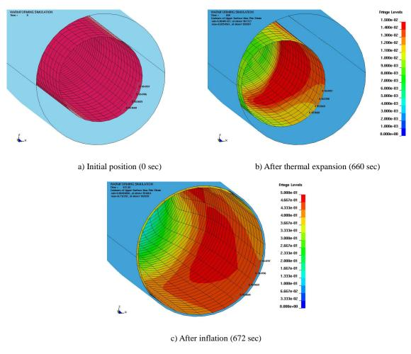
Figure 10: Strains at the lengthwise middle of the tube during warm forming
