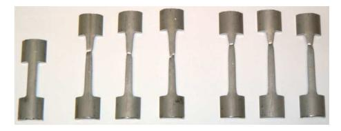
Figure 6: Intact (left) and tested 7075 aluminium alloy samples
