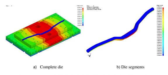
Figure 5: Temperature distribution in the heating die at the beginning of the second step
