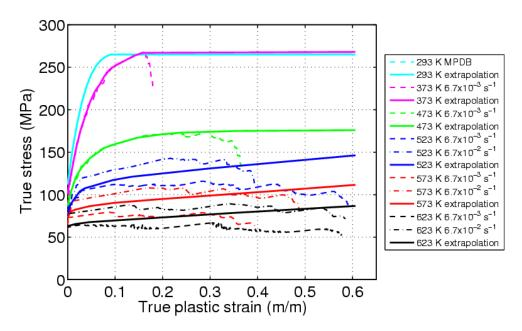
Figure 7: Measured and extrapolated curves for 7075 aluminium alloy at different temperatures
