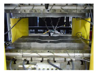
Figure 1: Heating die for warm tube forming
