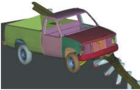
(c) Impact with steel box post, case 1
