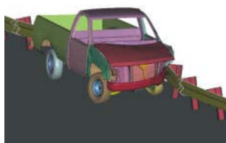
(b) Impact with Steel I-beam post
