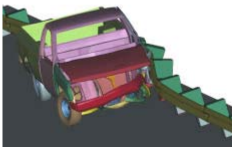
(a) Impact with wood posts
