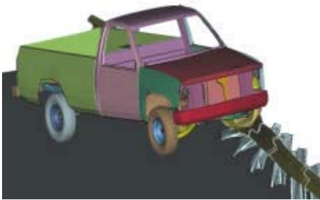
(e) Impact with Z-shape post, case 1
