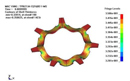
Figure 8 The uniform thickness distribution of pre form stage.
