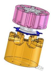
Figure 4 The pre-form stage Punch, Holder and Die CAD model.
