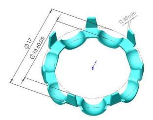
Figure 3 Dimension for miniature retainer with fingers.
