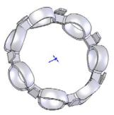
Figure 1 Small ball bearing with fingers for retainers clamped.
