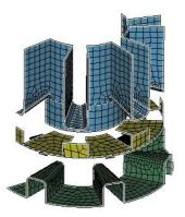
Figure 5 The pre-form stage Punch, Holder and Die mesh model.
