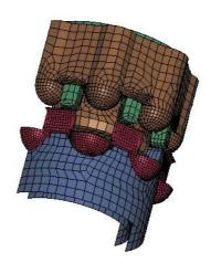
Figure 6 The finished-form stage Punch, Holder and Die CAD model.
