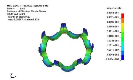
Figure 9 The plastic strain distribution of finished form stage.
