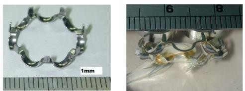
Figure 11 The finial stamping part and its cross section at the cage.
