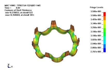
Figure 10 The thickness distribution of finished form.
