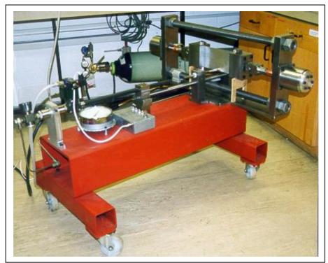
Figure 8: Fast crack growth loading device
