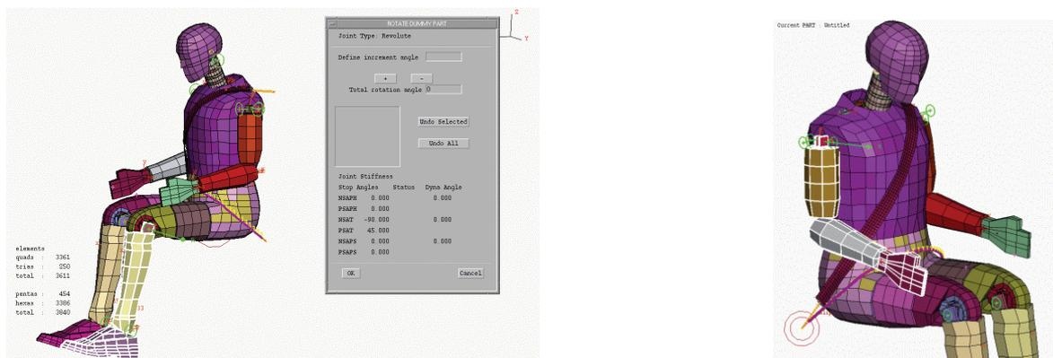
Figure 3.2: Positioning the dummy using ANSA 12.01
