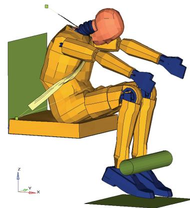
Figure 3.1: HyGee 25g Forward Impact Pulse
