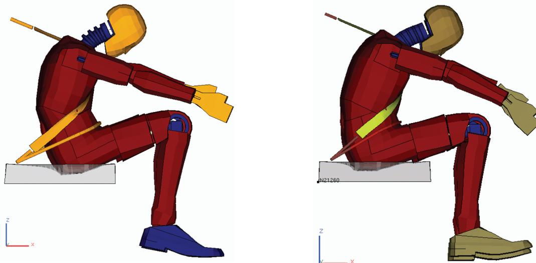
Figure 1.2: Comparison between dummy loading device behaviour with and without pre-positioning.
