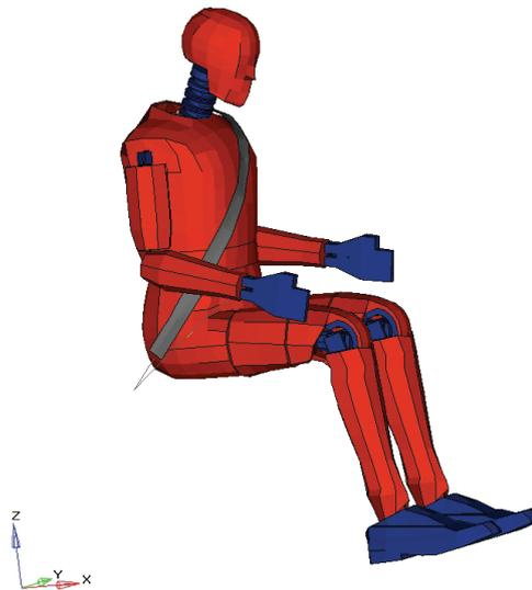
Figure 1.0: Hybrid III 95% Deformable Loading Device Dummy
