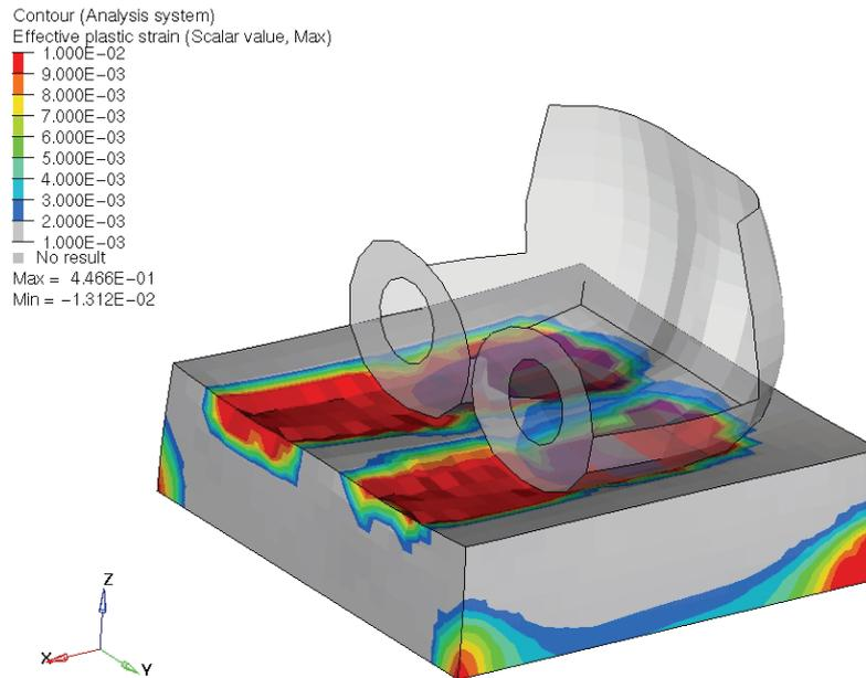
Figure 3.0: Stress initialisation in the seat cushion using LS-Dyna.
