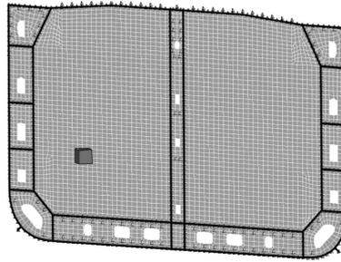
Figure 4 Connection of deformable and rigid parts, connection nodes are drawn in black.
