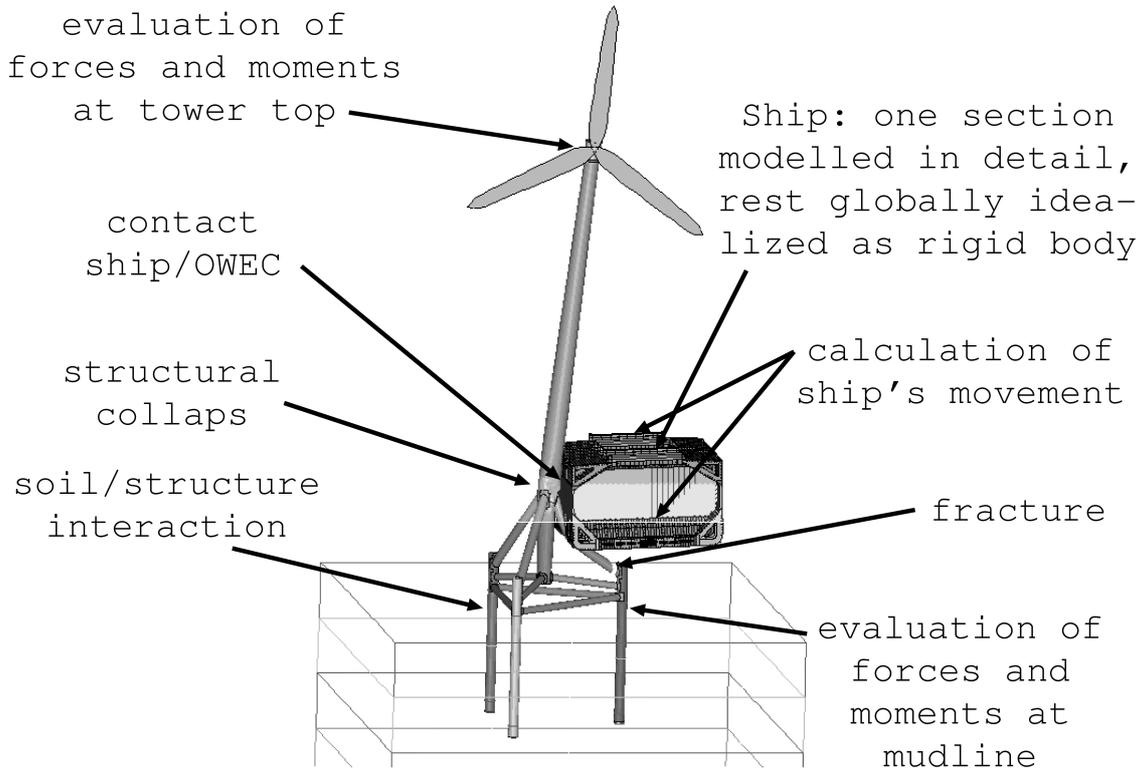
Figure 7: collision: input data, parameters, and output data
