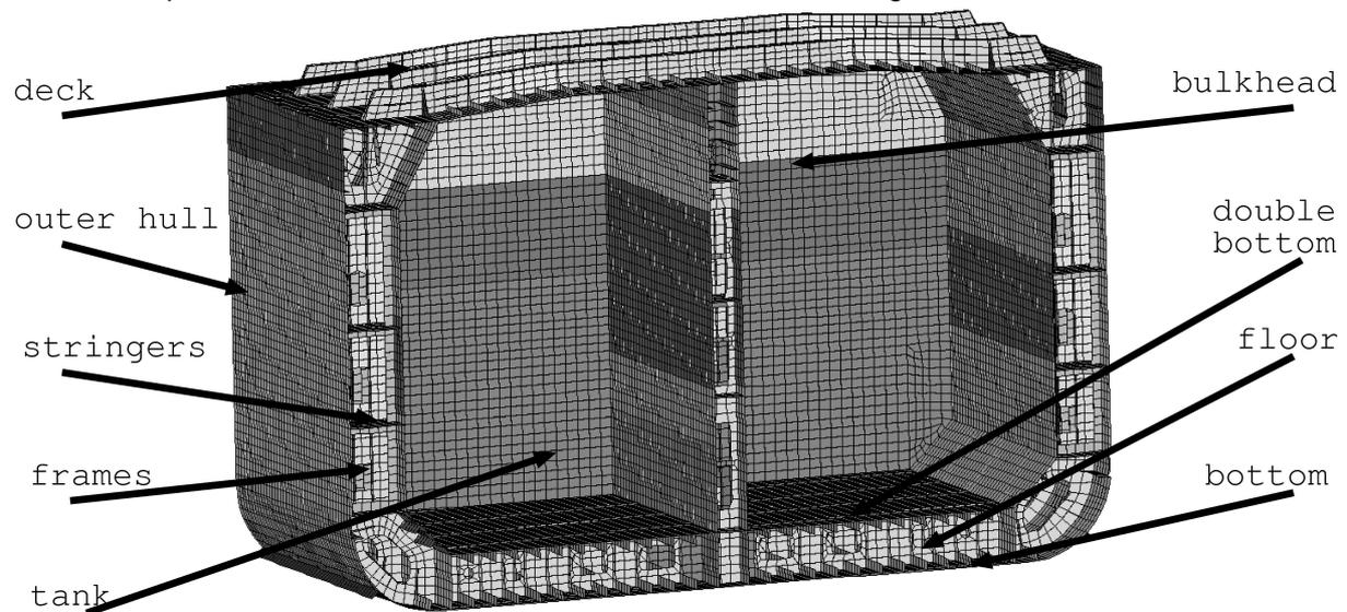
Figure 3 Section of a double hull tanker
