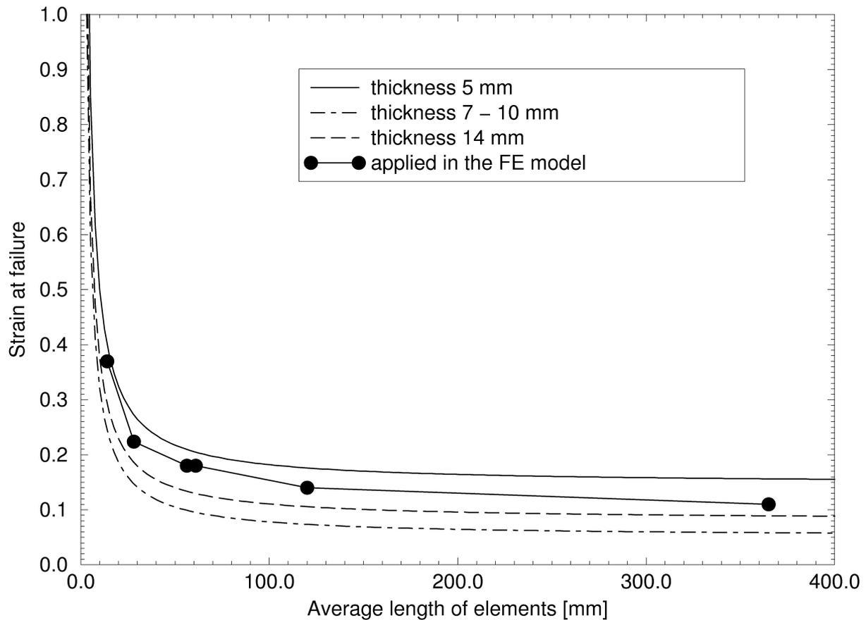
Figure 8 strain at failure depending on side length and gage of steel plate
