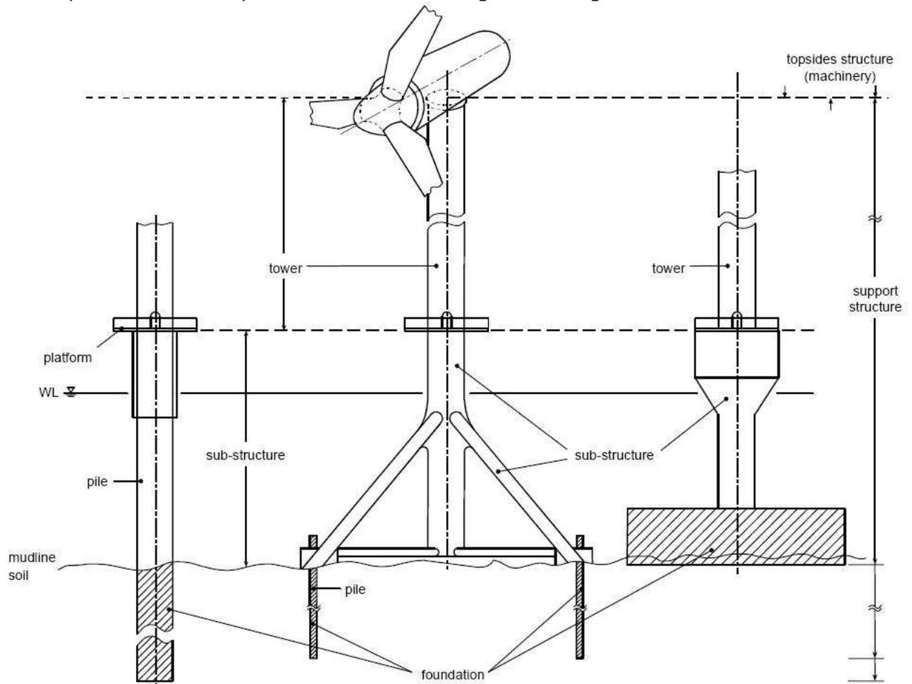
Figure 5 Definition of offshore wind turbine sections
