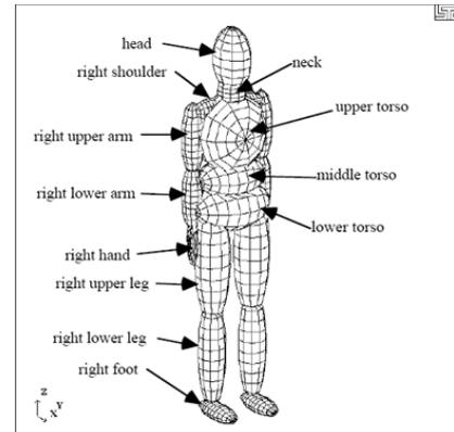
Figure 3: GEBOD Dummy Model (LS-Dyna manual)
