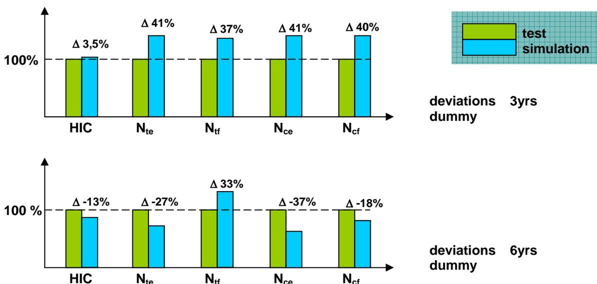
The deviations of the 3yrs dummy model concerning the HIC value are very small, so the HIC value can be used without doubt. For the NIJ value, all four deviations are rather high, but almost in the same range of 37-41%. So they can be used, too, by "calculating back" to the test results.
