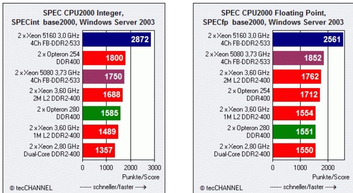
Fig. 3: Comparison of Intel Xeon and AMD Opteron based on Spec benchmark
