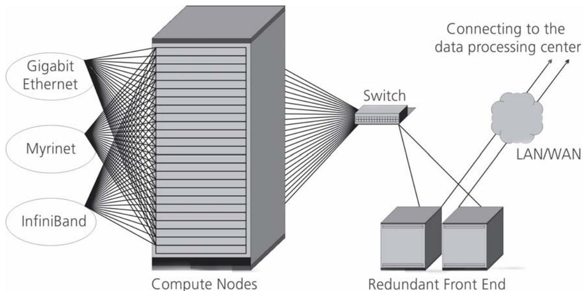
Fig. 2: Architecture of an HPC cluster in principle
