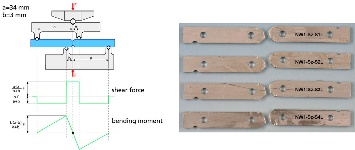
Fig. 3: schematic drawing of the modified losipescu shear test and shear specimens after test
