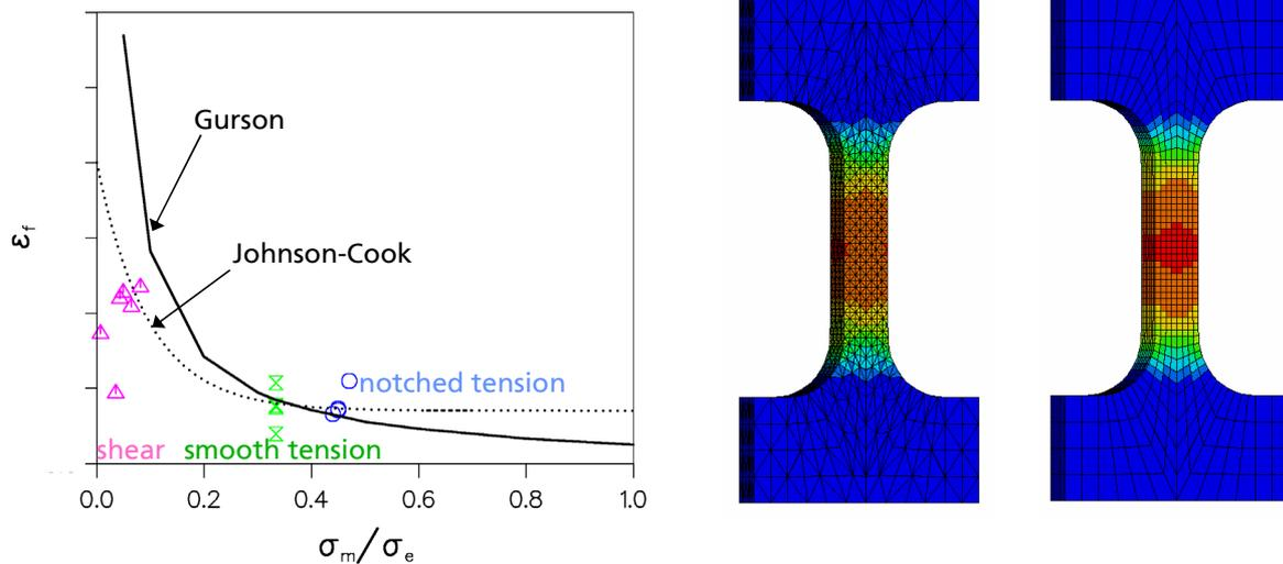
Fig. 9: plastic failure strain vs. stress triaxiality for the Gurson and Johnson-Cook models and contour plots of the Johnson-Cook damage variable  $D$  shortly before the onset of damage for smooth tensile specimens modelled with TET4 and HEX8 elements
