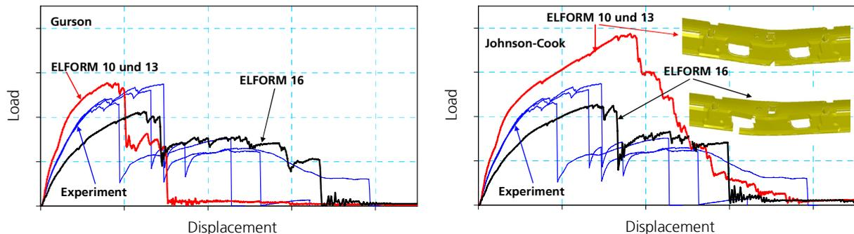
Fig. 13: load vs. displacement curves calculated with different element formulations for the Gurson model (left) and Johnson-Cook model (right) in comparison with the experimental results and damage pattern calculated with the Johnson-Cook model and ELFORM 16 (right)
