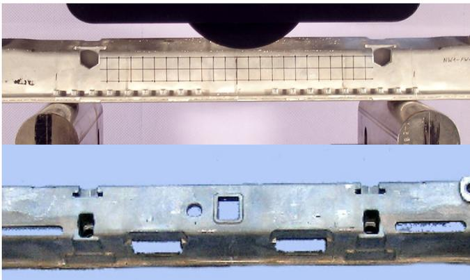
Fig. 8: geometry of a component and test setup for bending tests
