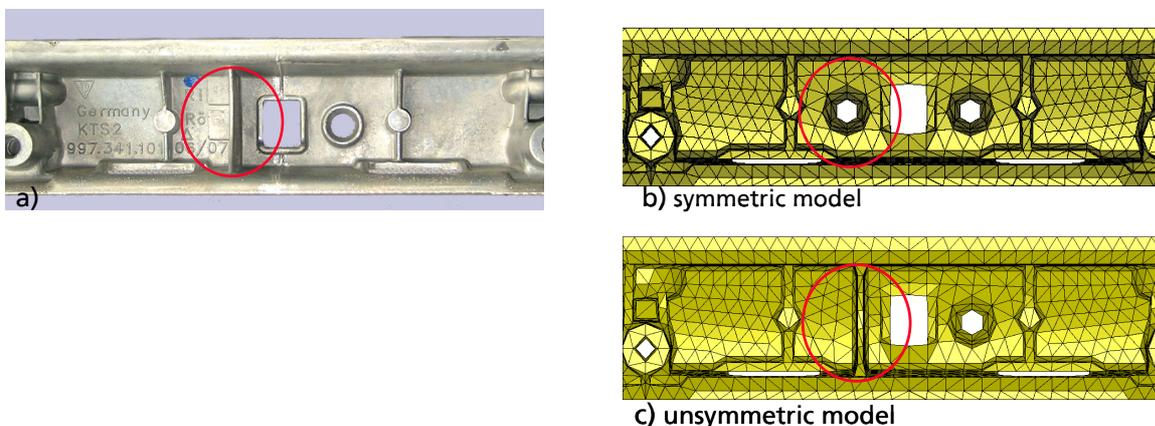
Fig. 10: a) component geometry of the centre section, b) and c) geometries of two different finite element models
