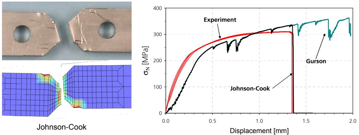
Fig. 5: comparison of fracture patterns and nominal stress vs. displacement curves between experiment and simulations for the Iosipescu shear tests
