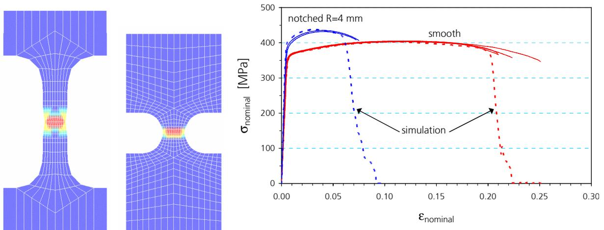
Fig. 4: contour plots of the Gurson damage variable  $f$  shortly before the onset of damage and comparison between the measured and simulated nominal stress vs. nominal strain curves for the tension tests
