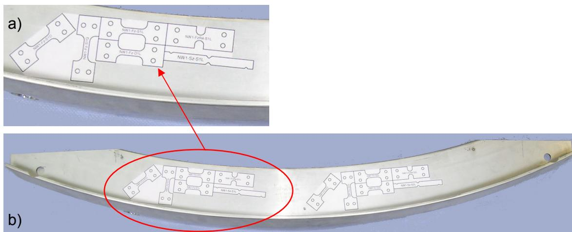
Fig. 1: a) one position of specimen extraction for material characterisation, b) geometry of the bumper
