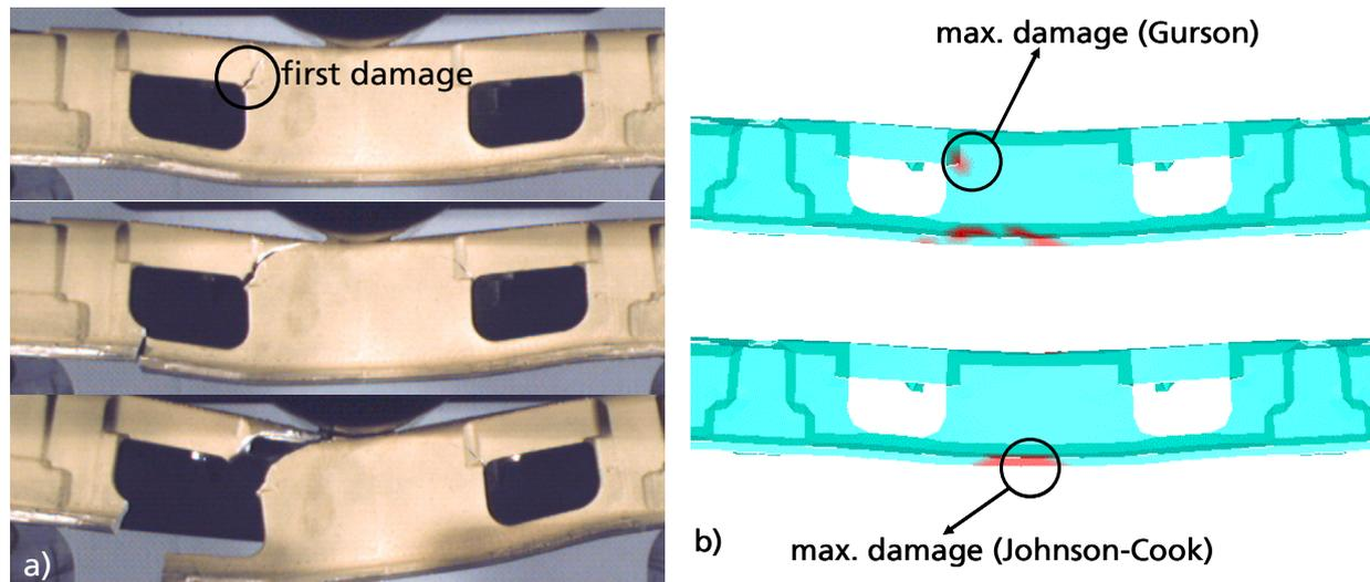
Fig. 12: a) development of damage during the bending test, b) distribution of the damage variables  $f$  (Gurson model) and  $D$  (Johnson-Cook model) before the onset of failure
