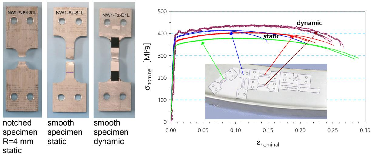
Fig. 2: smooth and notched flat tensile specimens after test and measured nominal stress vs. nominal strain curves for static and dynamic loading and for different specimen orientations (static loading)
