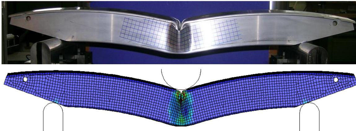
Fig. 7: bumper after three-point-bending-test and result of simulation (Gurson model)
