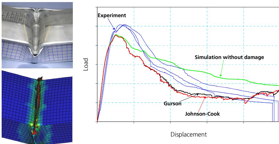
Fig. 6: damage pattern in experiment and simulation (Gurson model) and measured and calculated load vs. displacement curves for the three-point bending tests on the bumpers
