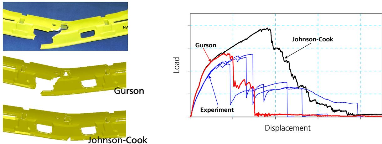
Fig. 11: damage pattern in experiment and simulations and measured and calculated load vs. displacement curves for the bending tests
