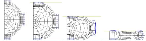
Fig. 6a: Deformation of the structure without failure of the adhesive
