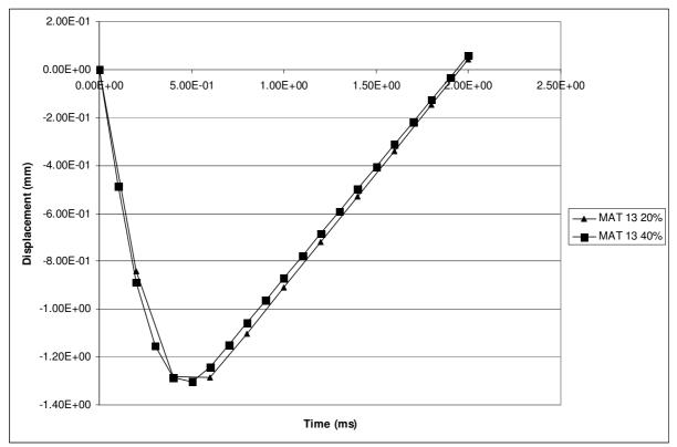
Fig. 11: Displacement for different values for the plastic failure strain
