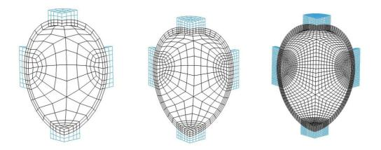
Fig. 4: FE-Model with a coarse, a medium sized and a fine mesh
