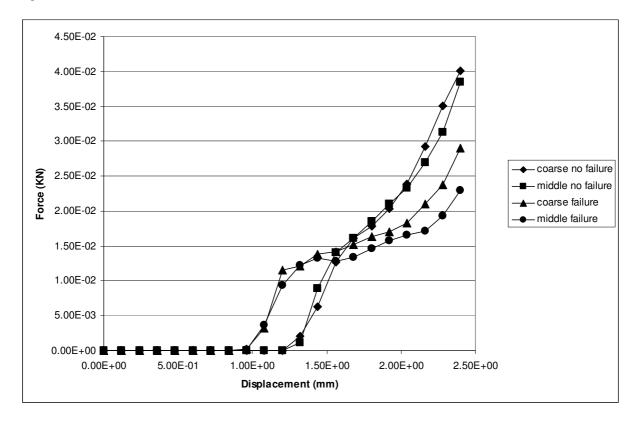
Fig. 7: Force-displacement diagram for different levels of mesh size and failure criteria.
