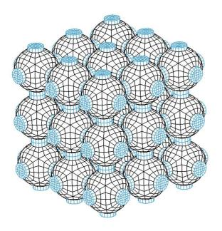
Fig. 3: Regular assembly of spheres as a 3D structure in a primitive cubic pattern
