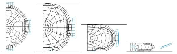
Fig. 6b: Deformation of the structure with failure of the adhesive
