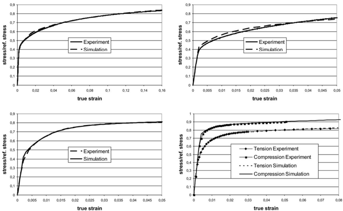
Fig. 2: Comparison of experimental and numerical results. Upper left: uniaxial tension in RD. Upper right: uniaxial compression in RD. Lower left: uniaxial compression in RD after 10% tensile pre-strain in RD. Lower right: uniaxial tension and compression in TD, respectively, after 10% tensile pre-strain in RD.
