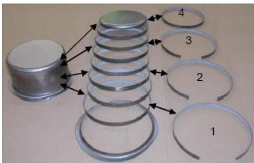
Fig.4: Ring splitting test on DC04 from [7].
