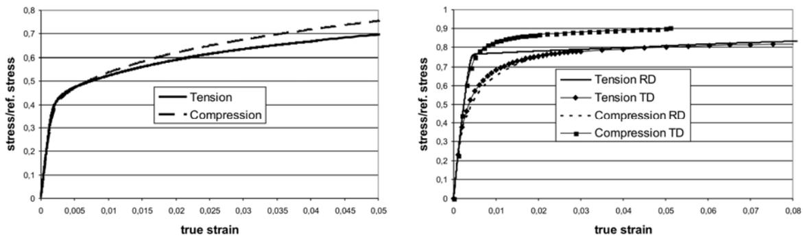
Fig. 1: Experimental results. Left: tensile and compressive yield curves in RD on the as-received material. Right: tensile and compressive yield curves after 10% tensile pre-strain in RD.
