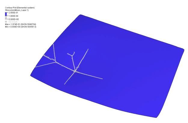
Figure 5: Improved laminated glass model respecting rupture with regular tria mesh
