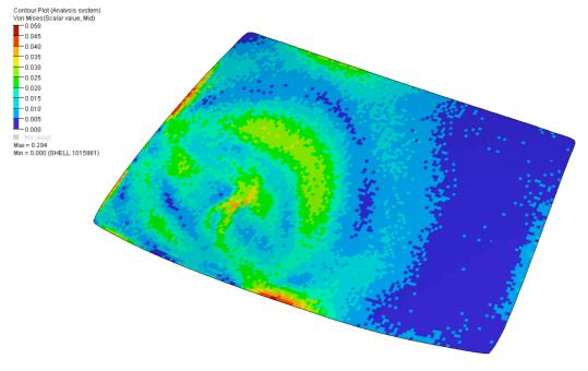
Figure 4: Simple elasto-plastic model with regular quad mesh
