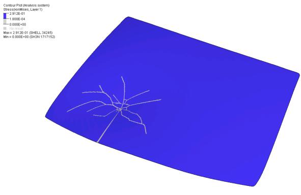
Figure 6: Improved laminated glass model respecting rupture with regular tria mesh
