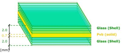
Figure 17: next step: shell-solid-shell model
