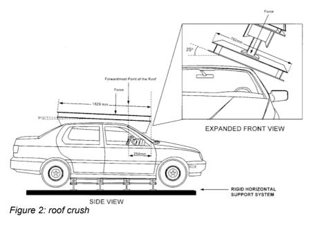
Because of respecting physical laminated glass properties the advanced model also improves the behaviour of the windscreen under quasi-static roof crush load case.
