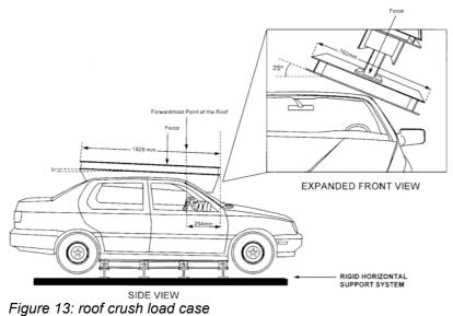
For roof crush load case the advanced laminated glass model show significant improvement of model predictability without any changes of the windscreen model used for head impact (see figure 14).
