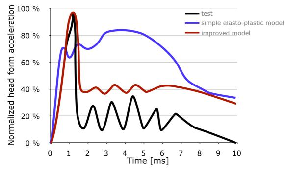
Figure 11: normalized head form acceleration over impact time
