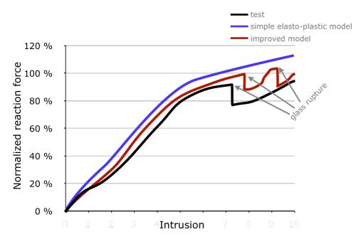
Figure 14: roof crush – normalized reaction force over intrusion
