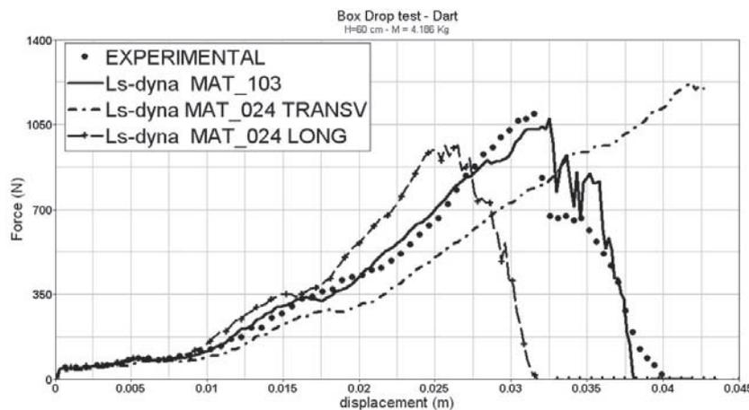
Fig. 7: Box drop test. Curves force displacement obtained with MAT\_103 (continuous line), compared to the curves obtained with isotropic modeling and the experimental curve (dots).
