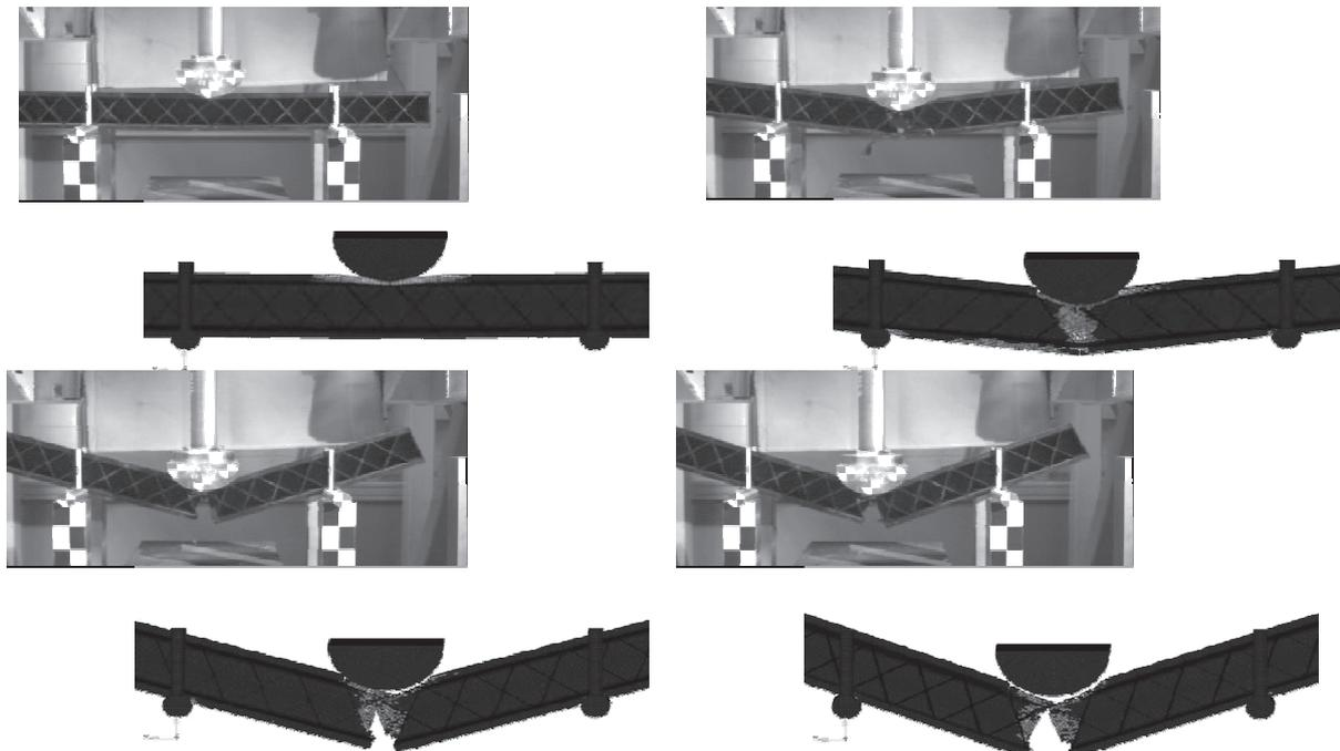
Fig. 11: Real and virtual deformation and failure behaviors of the ribbed beam at different times during the impact sequence. Images from testing courtesy of Faurecia Seatings.
