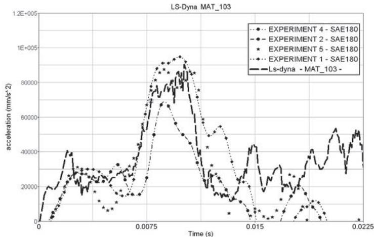
Fig. 10 : Curves of impactor acceleration vs. time: comparison between four experimental realizations and the simulation result for the impact test on the ribbed beam.
