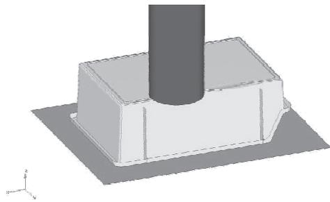
Fig. 8. Schematic representation of the not-instrumented drop test
