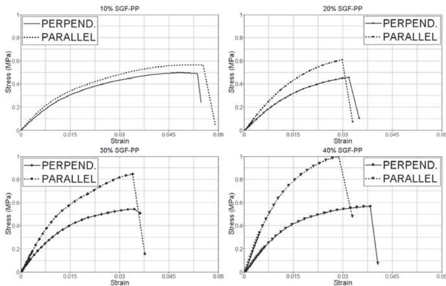
Fig. 1: SGF-PP curves stress-strain, measured on specimens cut from a plaque in the direction perpendicular and parallel to the flow lines. Examples include four different fiber percentages (10%, 20%, 30%, 40%). The stress values are normalized to the maximum value measured.
