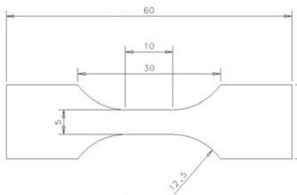
Fig. 3 T-bar specimen used for material characterization
