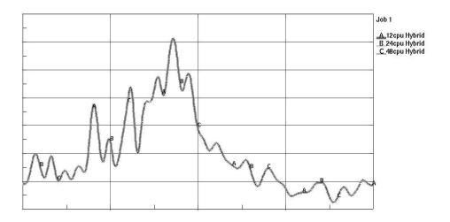
Job1 - vehicle deceleration response as measured at left rear sill
