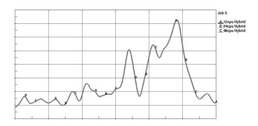
Job3 - vehicle deceleration response as measured at left rear sill
